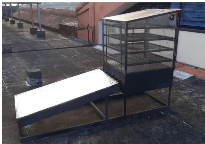
Figure 9. Mixed-mode solar dryer [48]
