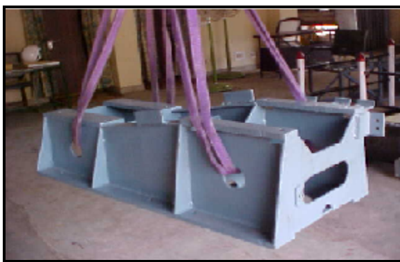
Fig 2: Experimental Set Up For Impact Hammer Test
