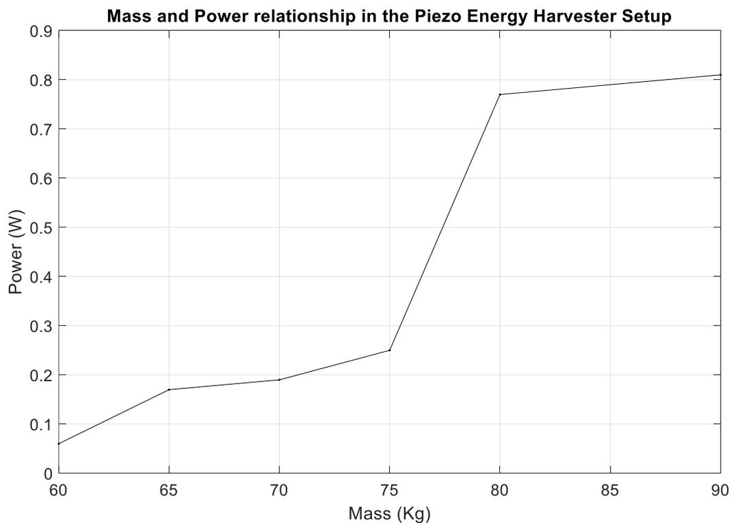
**Figure 6:** Power – Mass Relationship of the Energy Harvesting Device
