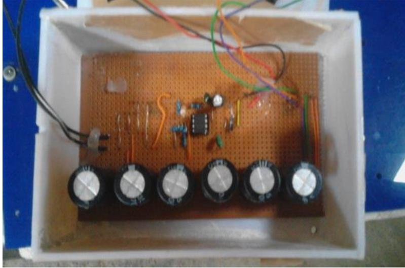
**Figure 3:** Energy harvesting prototype showing the capacitor bank
