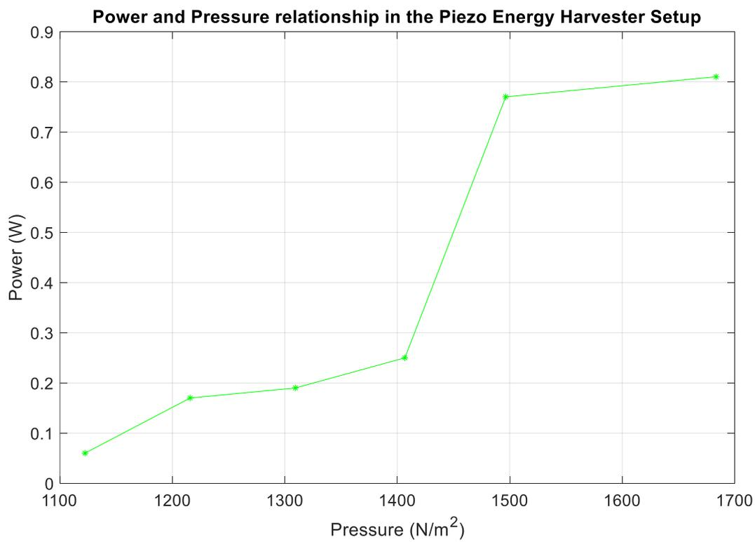
**Figure 7:** Power – Pressure Relationship of the Energy Harvesting Model
