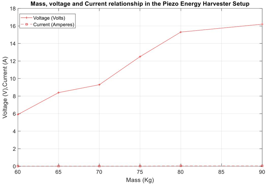
**Figure 8:** Current – Voltage Relationship of the Energy Harvesting Device
