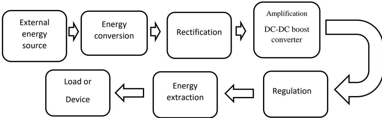
**Figure 1:** Block Diagram for the Realization of a Piezoelectric Energy Device
