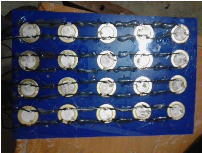
**Figure 2:** Energy Harvesting Prototype showing the arrangement of Piezo crystals
