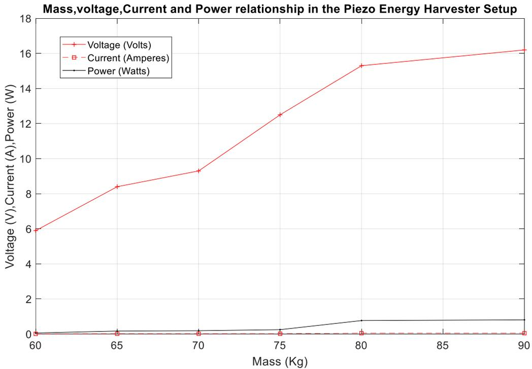
**Figure 9:** Power, Current, Voltage Relationship of the Energy Harvesting Device
