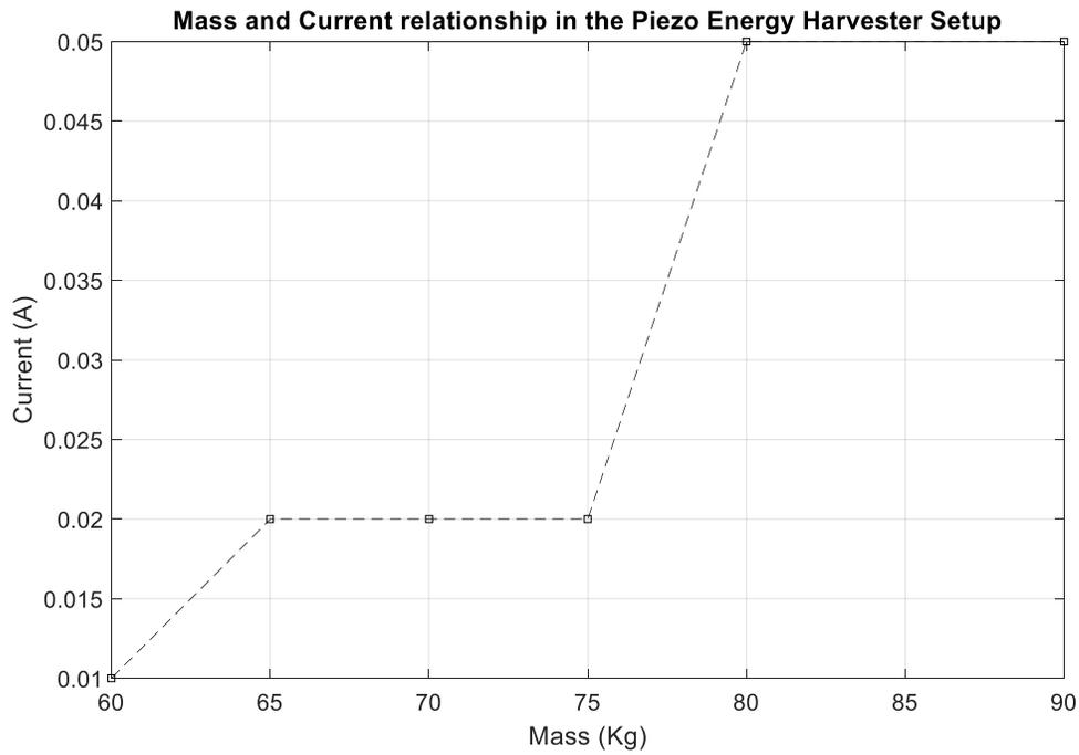
**Figure 5:** Current – Mass Relationship of the Energy Harvesting Device
