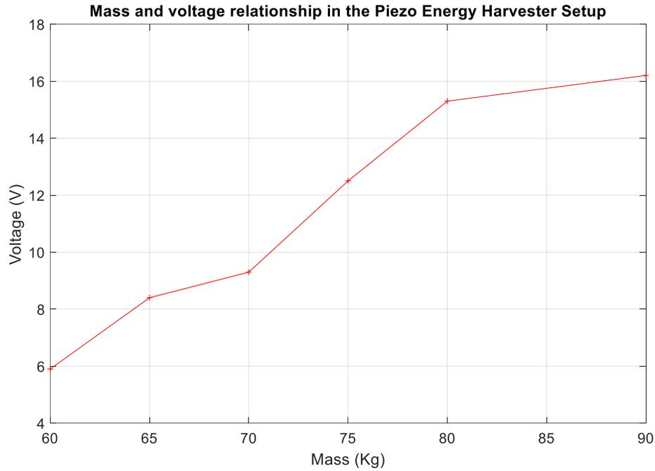
**Figure 4:** Voltage – Mass Relationship of the Energy Harvesting Device
