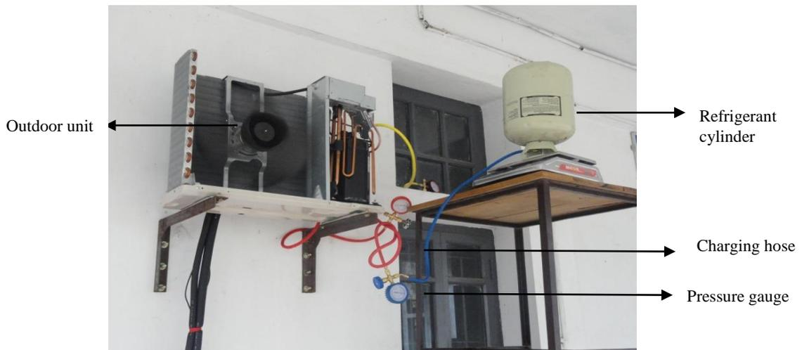
Figure 2. Experimental setup in laboratory and refrigerant charging system.
