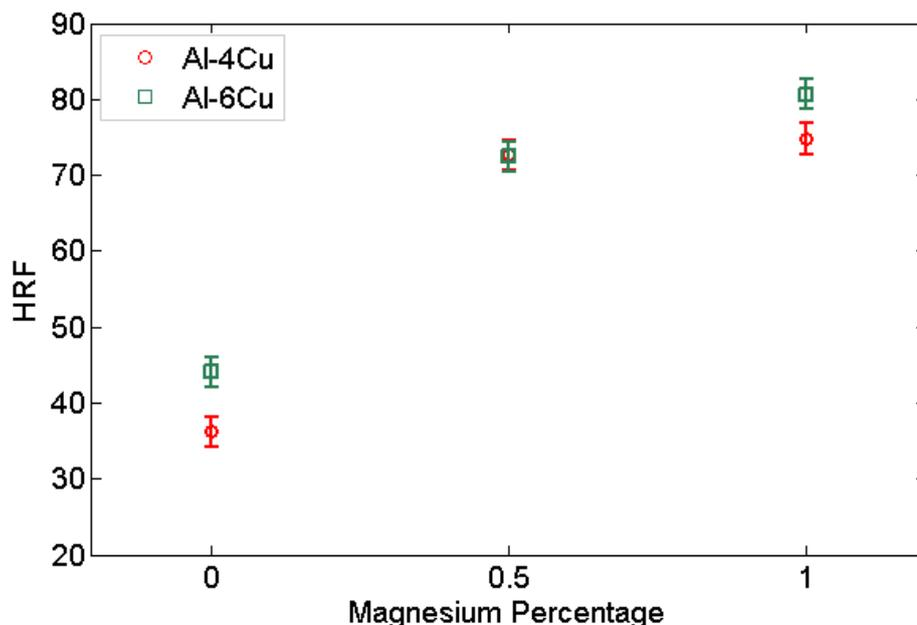
Figure 7. Hardness in HRF scale for both Al-4Cu and Al-6Cu alloys in the homogenized condition having different magnesium content.
