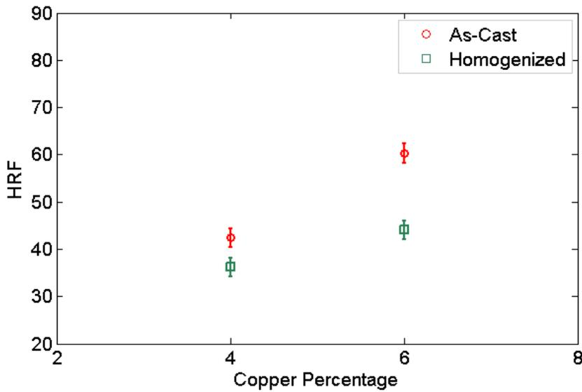
Figure 5. Hardness in HRF scale for both Al-4Cu and Al-6Cu alloys in the as-cast and homogenized condition
