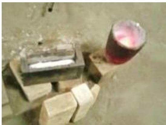
Figure 1. Casting of the alloys in a metal mold.
