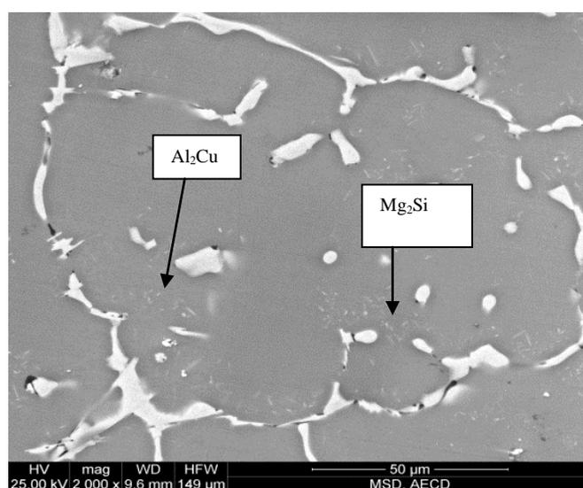
Figure 3. SEM micrograph of Al-6Cu-1Mg alloy. Identified phases are shown by arrows.
