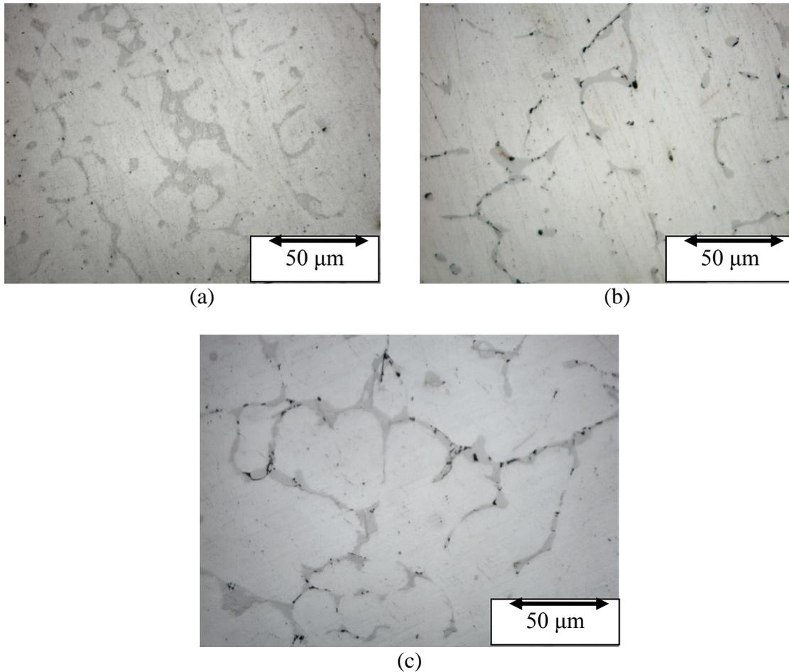
Figure 4: Optical micrographs showing microstructure of Al-6Cu alloys: (a) without any magnesium addition, (b) with 0.50 wt% magnesium addition, and (c) with 1 wt% magnesium addition
