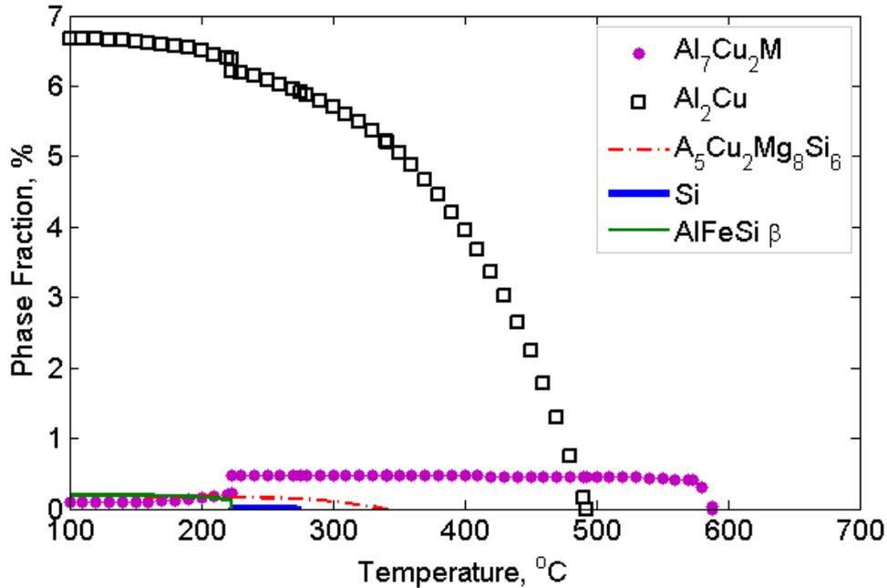
Figure 2. Predicted phase fractions for Al-4Cu alloy in the equilibrium condition in JMatPro software package
