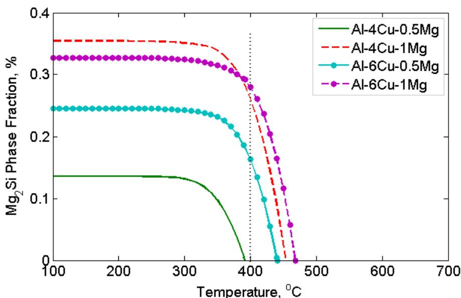
Figure 8. Fraction of  $Mg_2Si$  in Al-4Cu and Al-6Cu alloys at different temperatures
