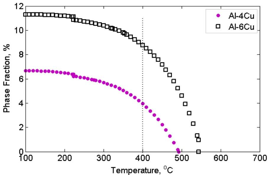
Figure 6. Fraction of  $Al_2Cu$  in Al-4Cu and Al-6Cu at different temperatures
