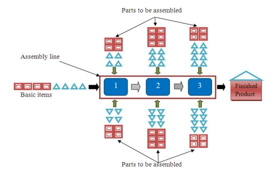
Figure 7. Multi-model assembly (adapted from Boysen et al. (2008)).
