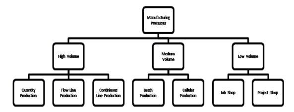
Figure 1. Decomposition of manufacturing processes.
