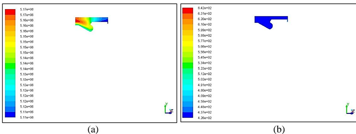
Figure 12. Pressure and temperature contours at crank angle (a) 372 degree and (b) 364 degree, respectively for 10WCOBD+10PSBD+80D+6lpm H<sub>2</sub>.
