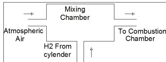
Figure 3. Mixing chamber of hydrogen and air.
