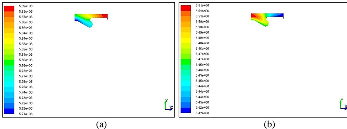
Figure 11. Pressure contour at crank angle (a) 352 degree and (b) 364 degree for 10WCOBD+10PSBD+80D+6lpm H<sub>2</sub>.
