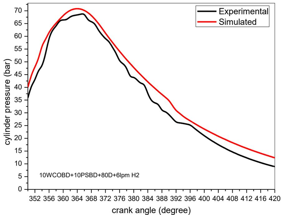
Figure 10. Comparison of simulated and experimental values of peak in-cylinder pressures against crank angles for 10WCOBD+10PSBD+80D+6lpm H<sub>2</sub>.
