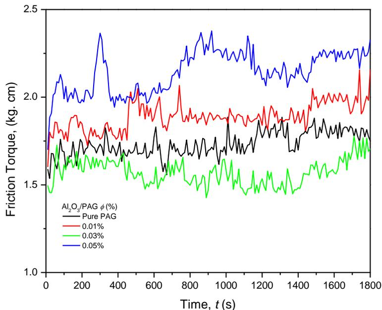
Figure 6. Friction torque evaluation of nanolubricants with time
