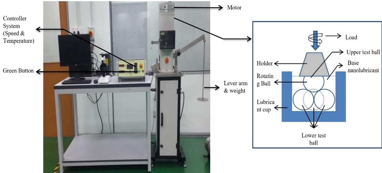
Figure 2. Tribology test using the Koehler four-ball tribo tester
