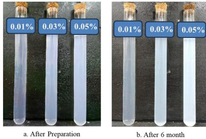
Figure 3. The visual photograph evaluation of Al<sub>2</sub>O<sub>3</sub>/PAG ND12 nanolubricants
