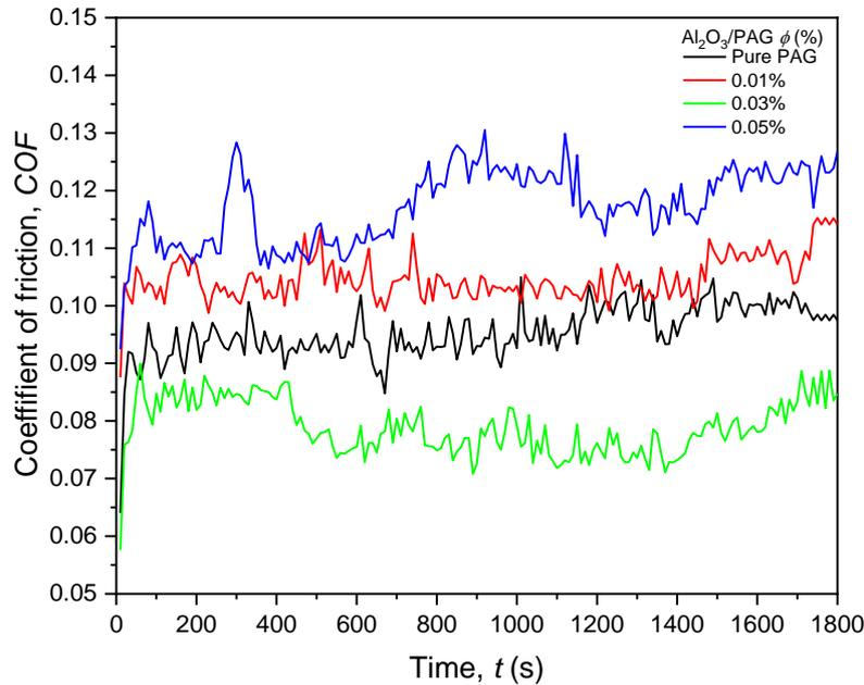
Figure 7. COF evaluation of nanolubricants with time
