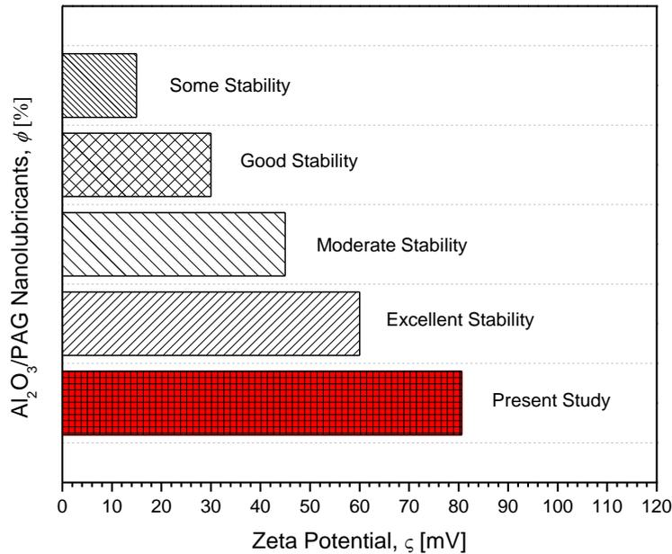
Figure 5. The zeta potential evaluation of  $\text{Al}_2\text{O}_3/\text{PAG}$  nanolubricants
