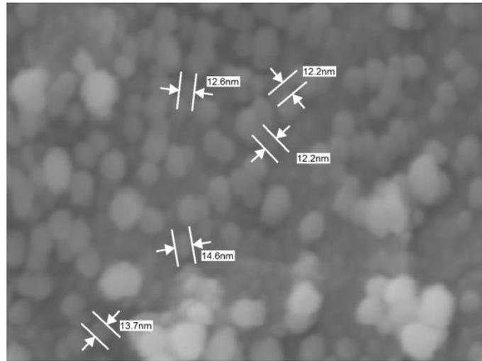
Figure 1. FESEM imaging for Al<sub>2</sub>O<sub>3</sub>/PAG ND12 nanolubricants
