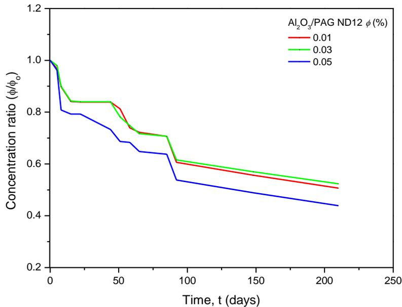
Figure 4. The concentration ratio of nanolubricants with sedimentation time
