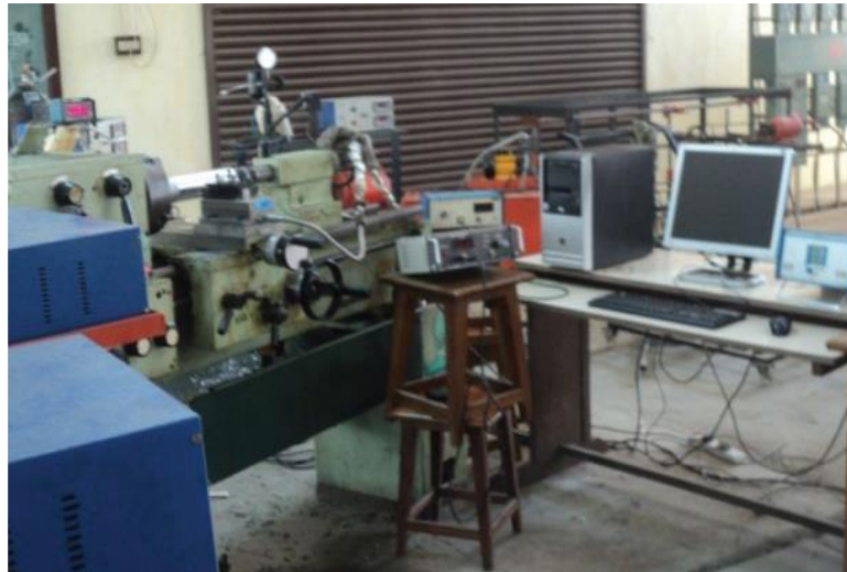
Figure 2. Kirloskar Turnmaster-35 all-g geared lathe for turning process
