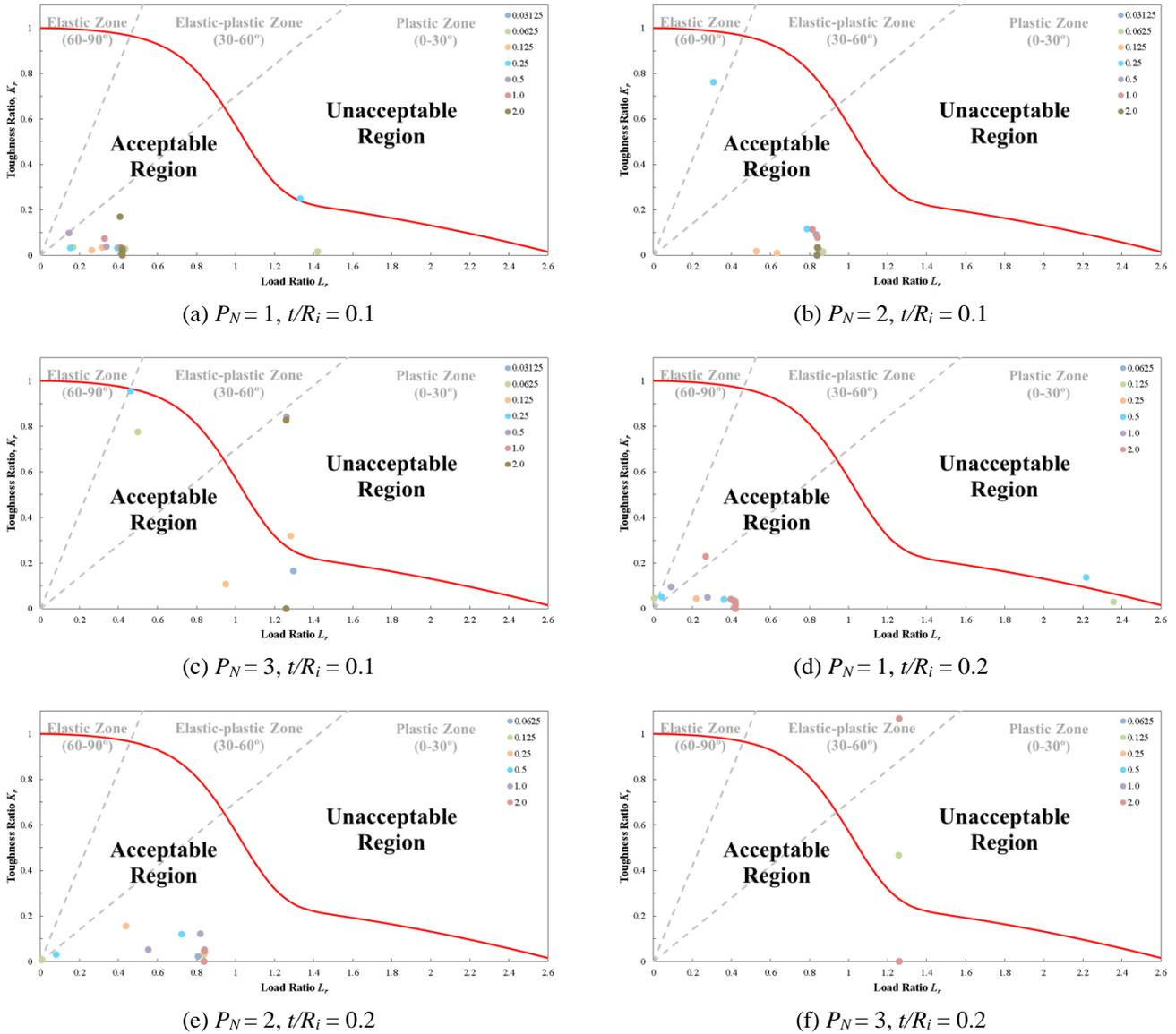
Figure 12. Assessment points for flaw sizes at different  $P_N$  and  $t/R_i$ , along with crack length  $a/c$  (a-b-c-d-e-f);
