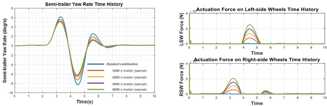
Figure 4. Open-loop performance of active auxiliary axle using truckSIM nonlinear model a) yaw rate performance in single lane change, b) actuator force on the right side (RSW) and left side (LSW) wheels
