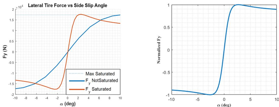
Figure 3. Tire modeling for improved lateral performance. a) Tire model in truckSIM for modified and original models. b) corresponding normalized lateral force against slip angle for MF model
