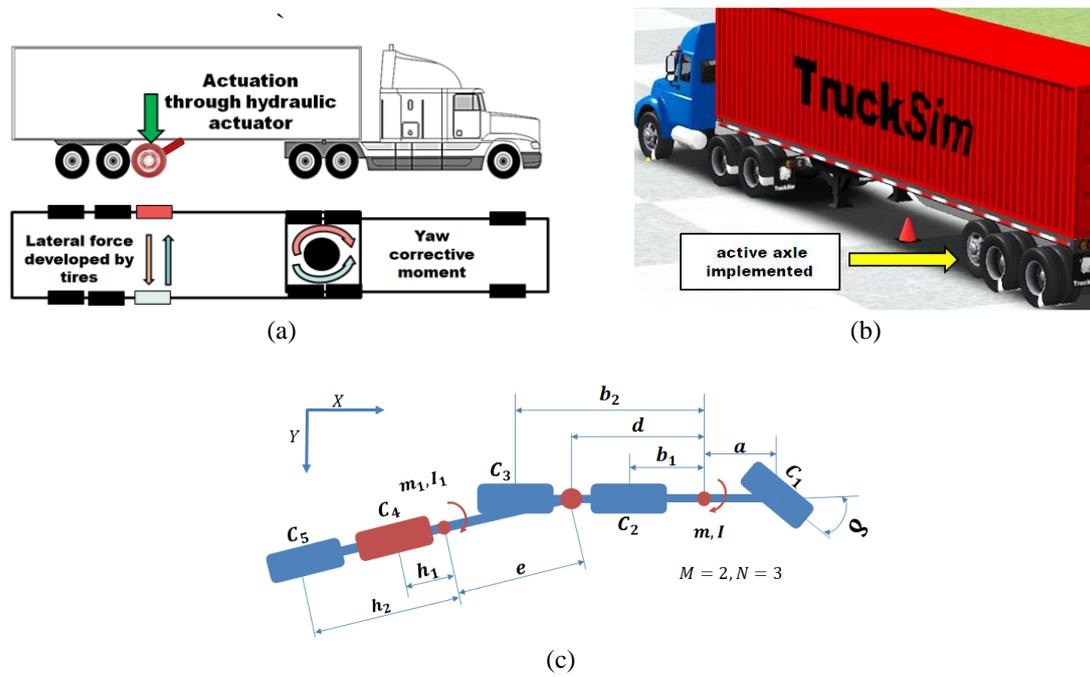
Figure 1. (a) The concept of proposed active auxiliary and development of corrective yaw moment (b) The five-axle nonlinear model in truckSIM equipped with an auxiliary axle, (c) mathematical yaw plane model to represent active auxiliary axle
