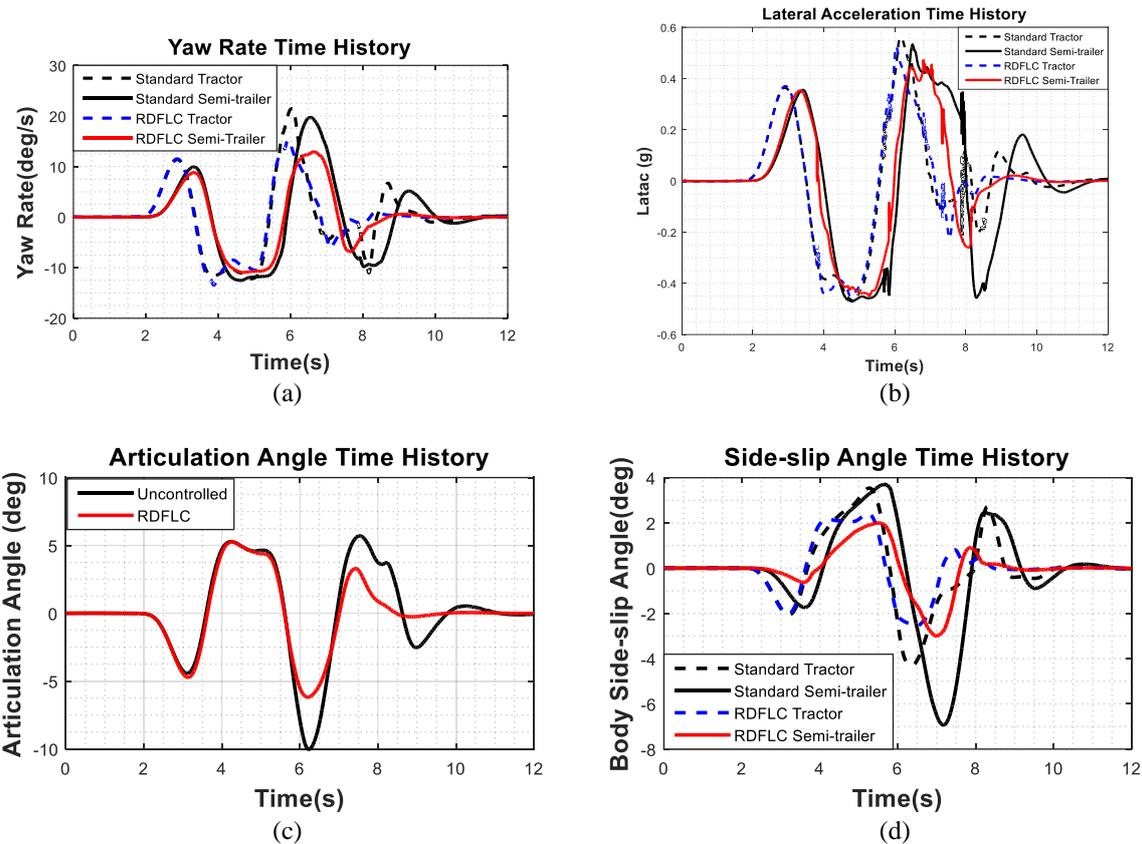
Figure 7. The effect of active axle intervention using a fuzzy logic controller in a double lane change maneuver with 7000kg of payload at 8000mm behind hitch point location (a) yaw rate, (b) lateral acceleration, (c) vehicle body side slip angle and (d) articulation angle
