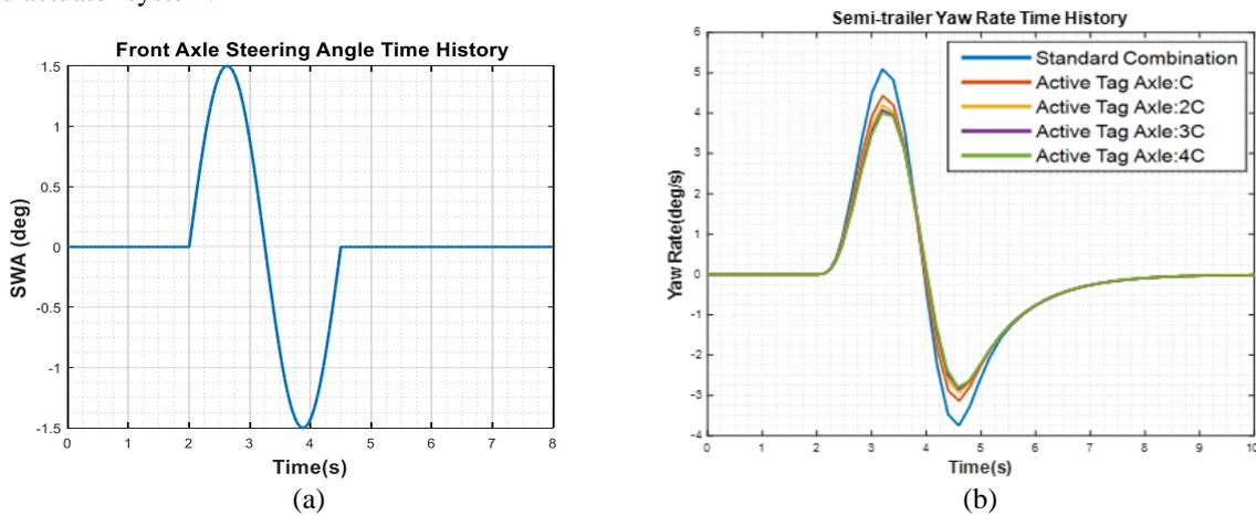
Figure 2. (a) Road wheel steering angle in open-loop single lane change maneuver, (b) Semi-trailer yaw rate response at 90km/h and 1.5 degrees of road wheel steering angle for different values of cornering stiffness of active axle
