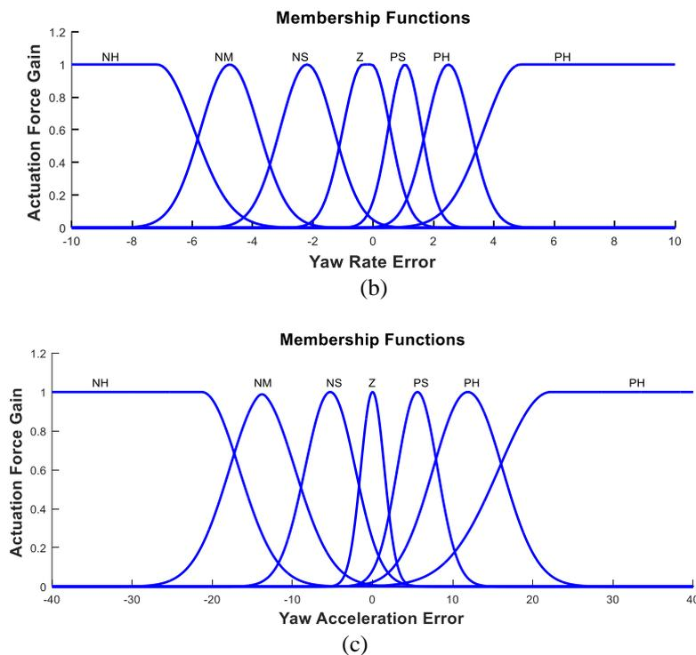
Figure 5. (a) Control system structure for active auxiliary axle (b) Membership functions of the yaw rate error (c) Membership functions of the error yaw acceleration error
