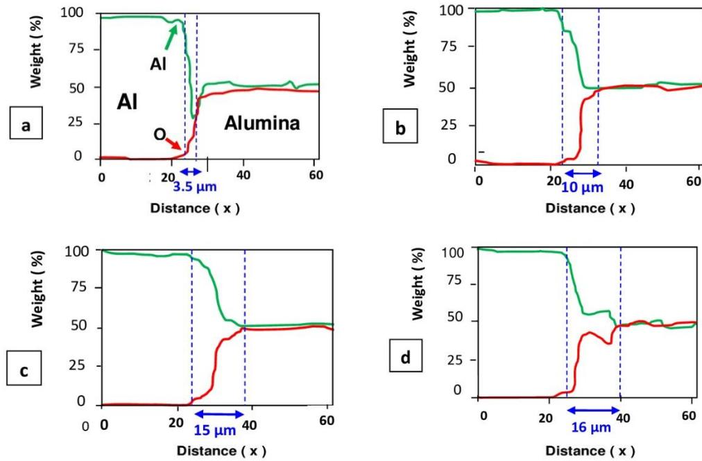
Figure 7. EDS analysis along welded alumina/Al 6060 alloy at 600°C for different bonding times (a) 2 min, (b) 3 min, (c) 4 min, and (d) 5 min
