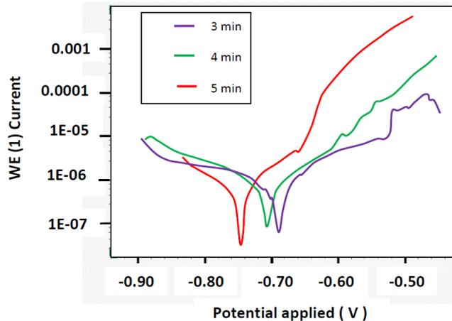
Figure 10. The polarization curves of the bonded alumina/Al 6060 alloy at 600°C for different bonding times (a) 3 min; (b) 4 min, and (c) 5 min
