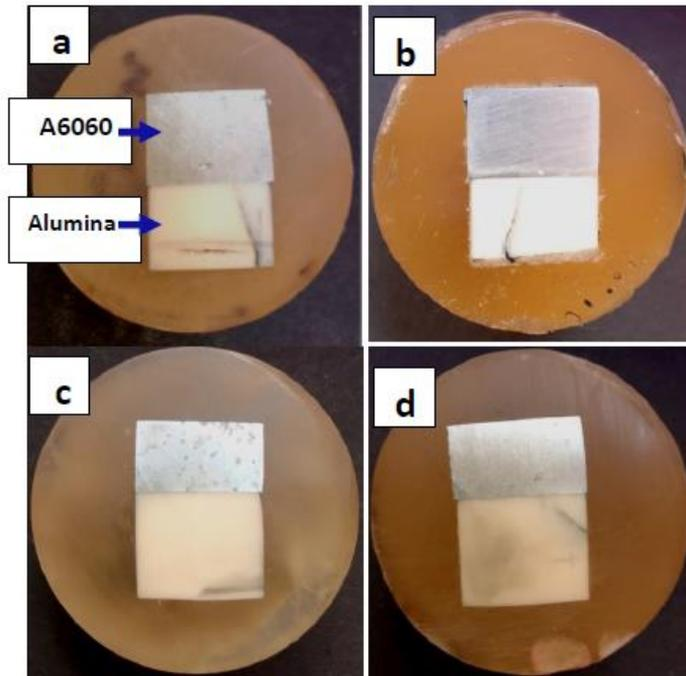
Figure 2. Samples obtained by solid state diffusion bonding at 600°C of alumina with aluminum 6060 alloy by solid state diffusion method for different times(a): 2 min, (b): 3 min, (c): 4 min, and (d): 5 min
