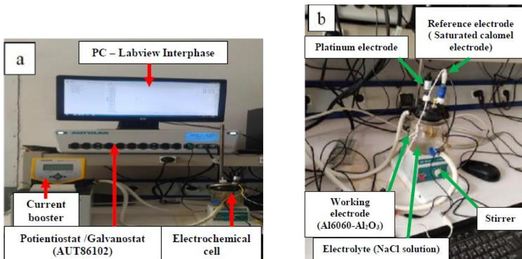
Figure 3. (a) AUTOLAB galvanostat potentiostat, (b) arrangement of electrodes
