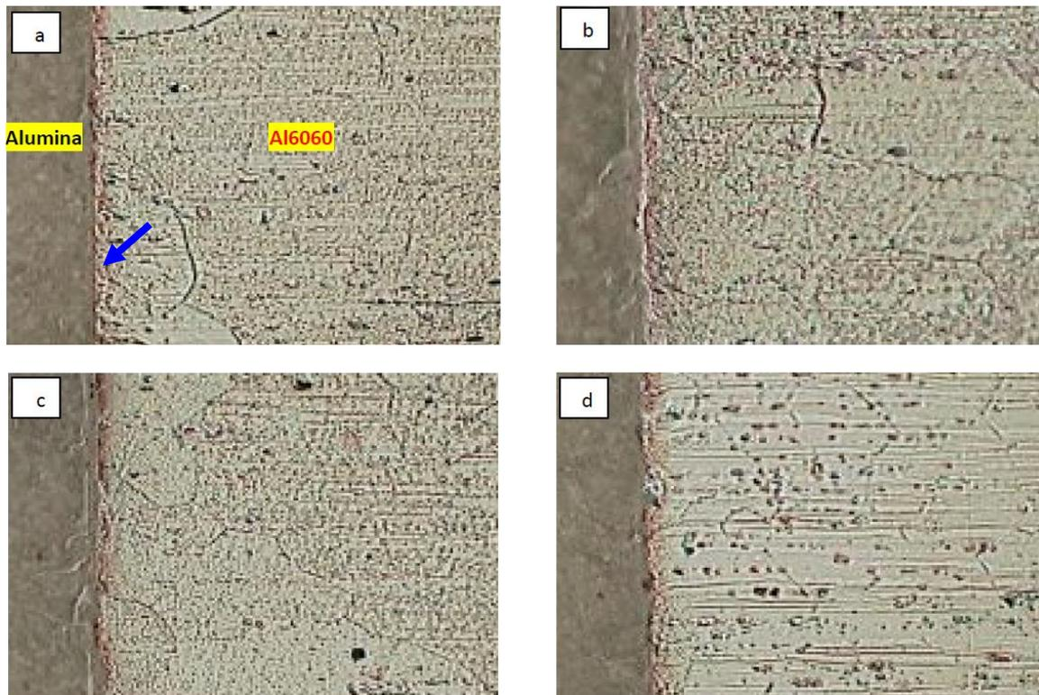
Figure 6. Microstructure evolution of the bonded interface alumina/Al 6060 alloy at 600°C for different bonding times (a) 2 min, (b) 3 min, (c) 4 min, and (d) 5 min
