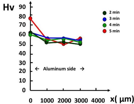
Figure 9. Hardness curves of bonded alumina/Al 6060 alloy at 600°C for different bonding times (a) 2 min, (b) 3 min, (c) 4 min, and (d) 5 min
