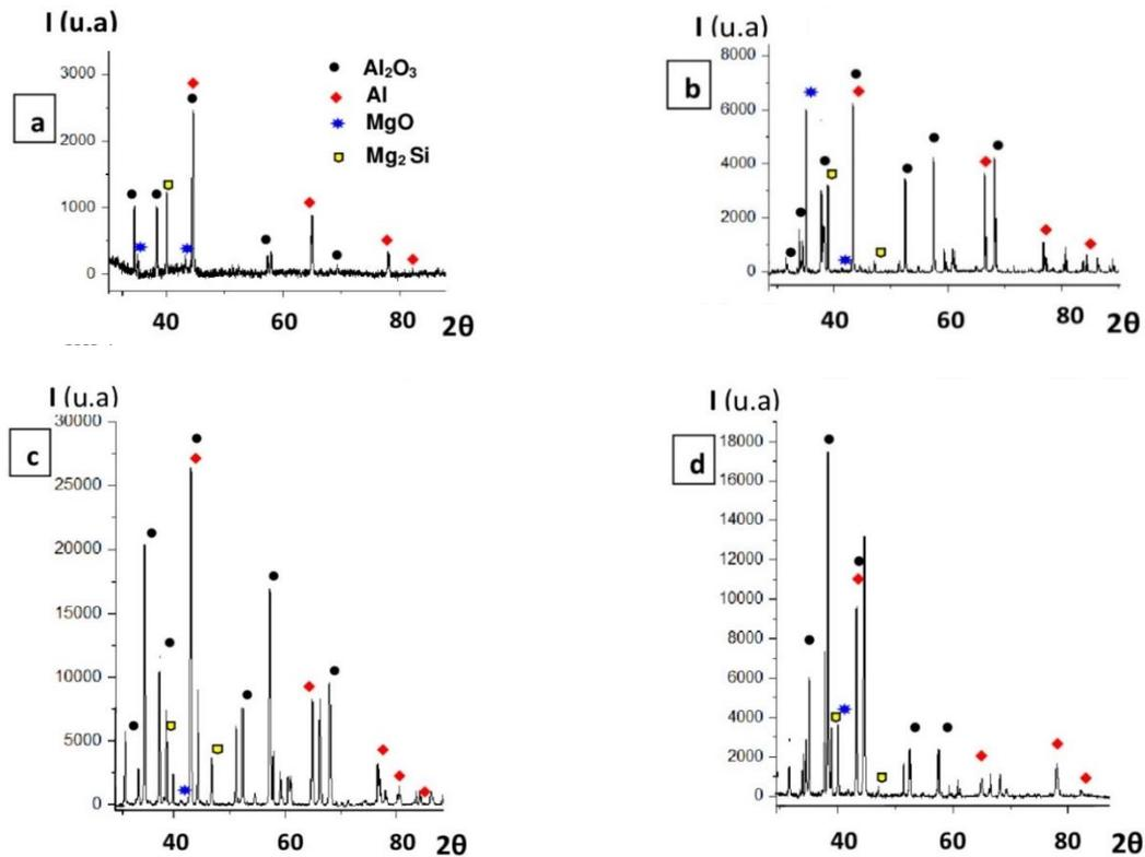
Figure 8. X-ray diffractograms of the bonded alumina/Al 6060 alloy at 600°C for different bonding times (a) 2 min, (b) 3 min, (c) 4 min, and (d) 5 min
