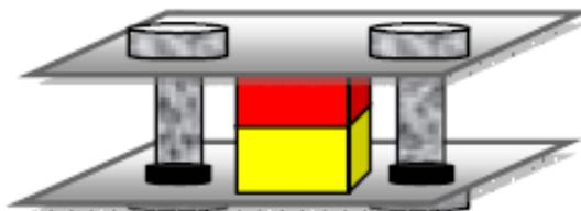
Figure 1. Solid-state diffusion bonding configuration applied for joining alumina to Al 6060 alloy
