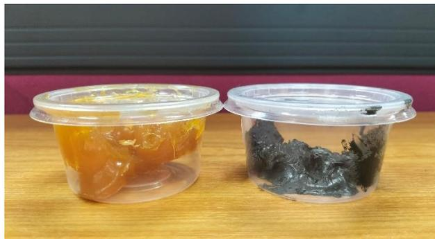
Figure 2. Comparison between lithium grease (left) and MRG (right)
