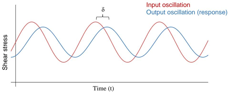
Figure 1. Schematic of phase angle measurement in oscillatory rheological experiments
