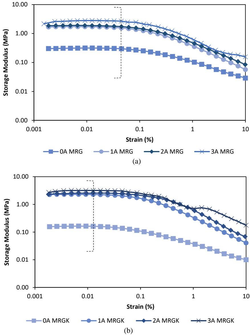
Figure 6. Storage modulus results for (a) MRG (b) MRGK after one year. Line marker shows the extent of LVE region
