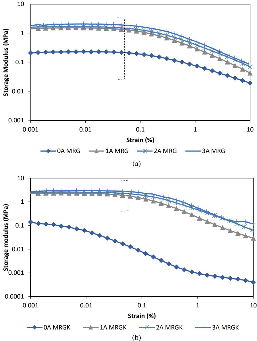
Figure 5. Storage modulus results for freshly synthesized (a) MRG (b) MRGK. Line marker shows the extent of LVE region
