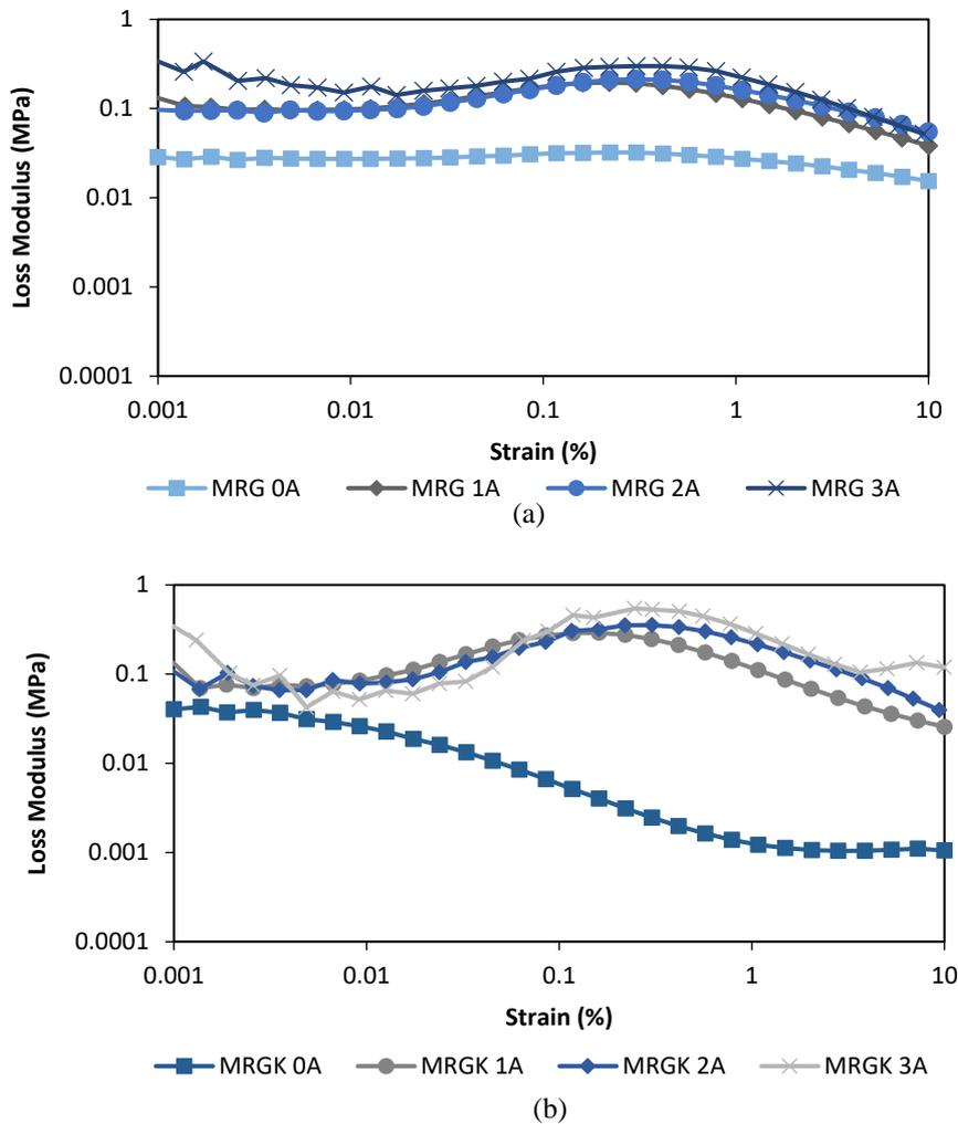
Figure 7. Loss modulus results for freshly synthesized (a) MRG (b) MRGK
