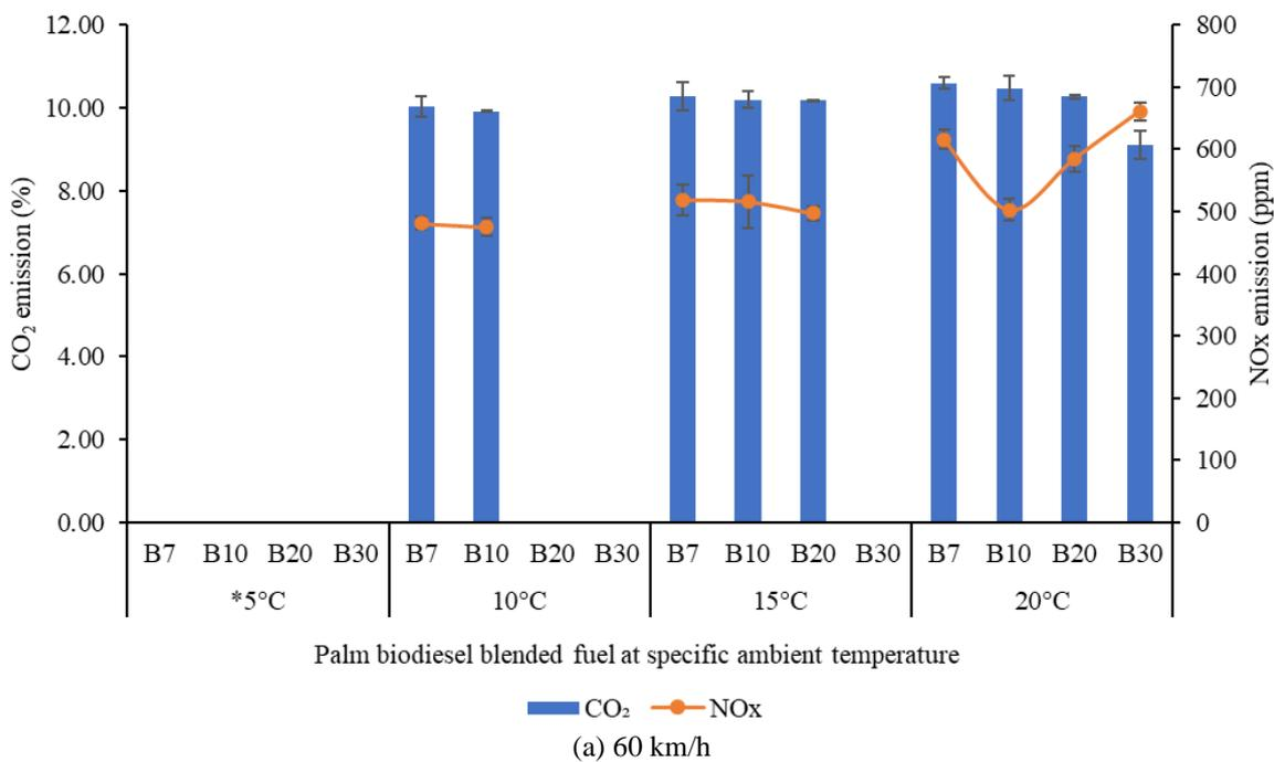
Figure 8. Effect of engine-out emissions of CO<sub>2</sub> and NO<sub>x</sub> at full load steady-state condition at (a) 60 km/h
