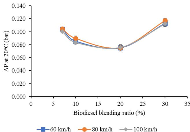
Figure 7. Pressure drop across the fuel filter at 20 °C under full load steady-state condition
