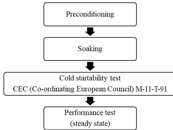
Figure 1. Cold test procedure
