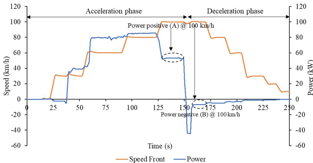
Figure 3. Example of engine power measurement under steady-state full load condition at cold ambient temperature
