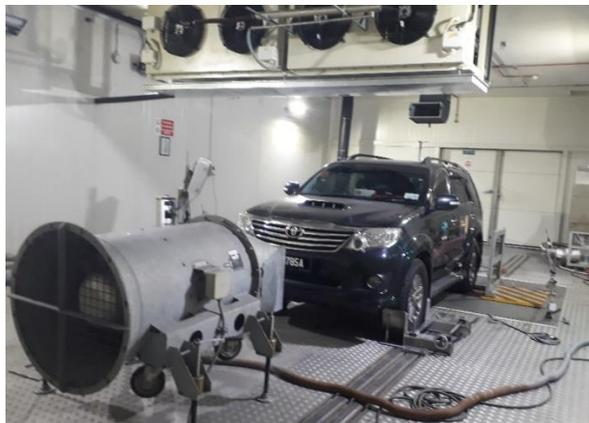
Figure 1. Cold chamber with the chassis dynamometer and the vehicle used in the study
