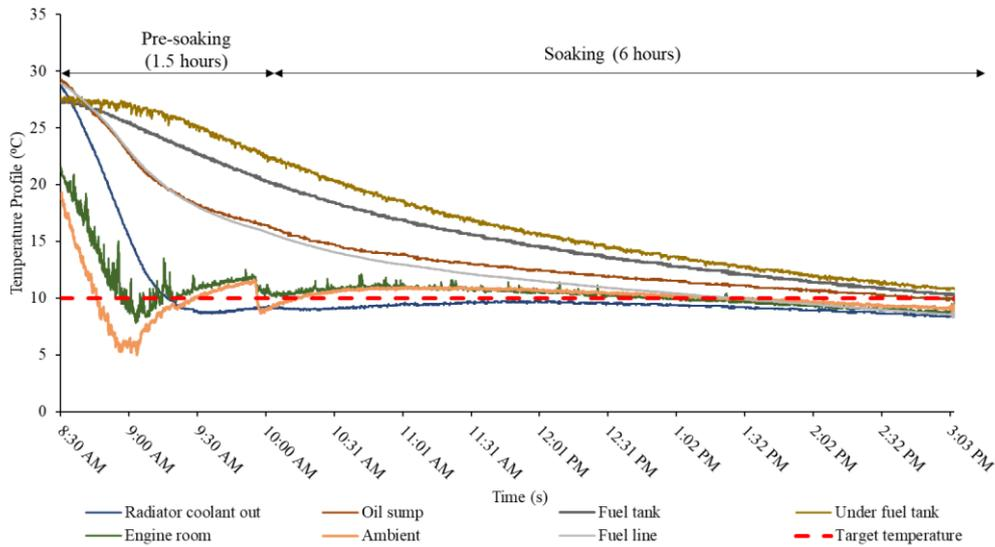
Figure 2. Temperature profile for soaking of B7 at 10 °C
