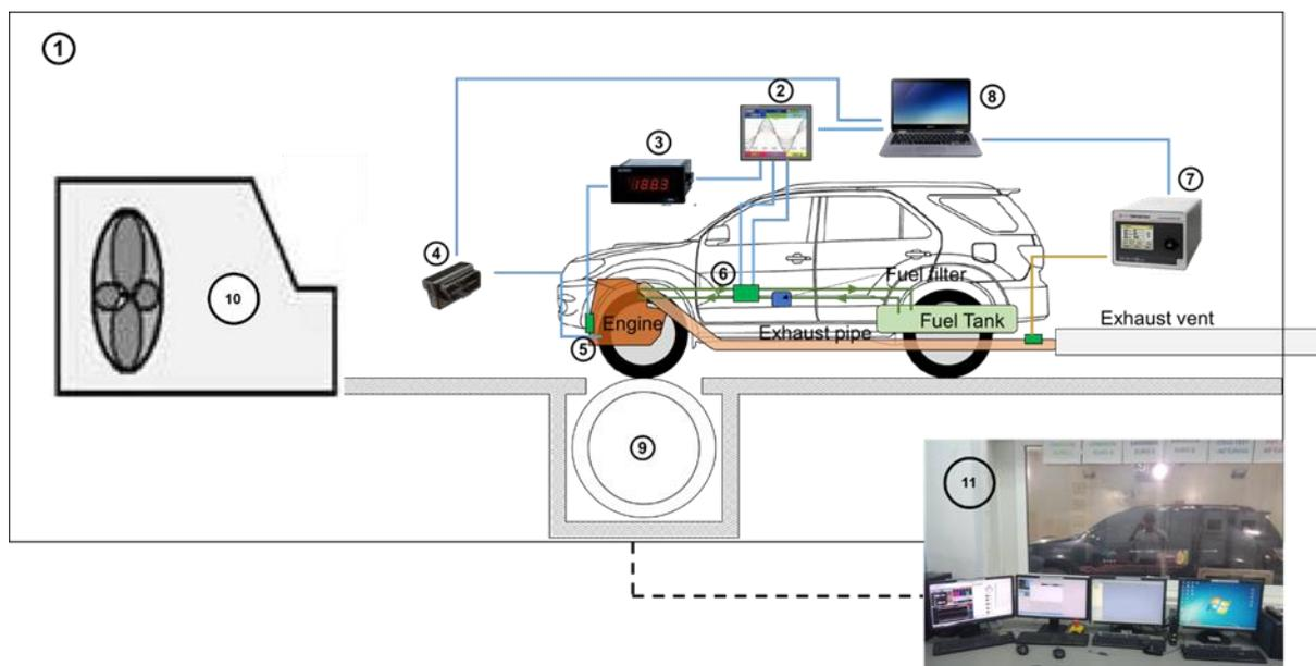
Figure 2. Experimental setup for cold performance test (1: cold chamber, 2: data logger, 3: counter (tachometer), 4: OBDII data logger, 5: IR sensor (tachometer), 6: fuel flow meter, 7: emission gas analyzer, 8: laptop, 9: chassis dynamometer, 10: wind simulator, and 11: control room)
