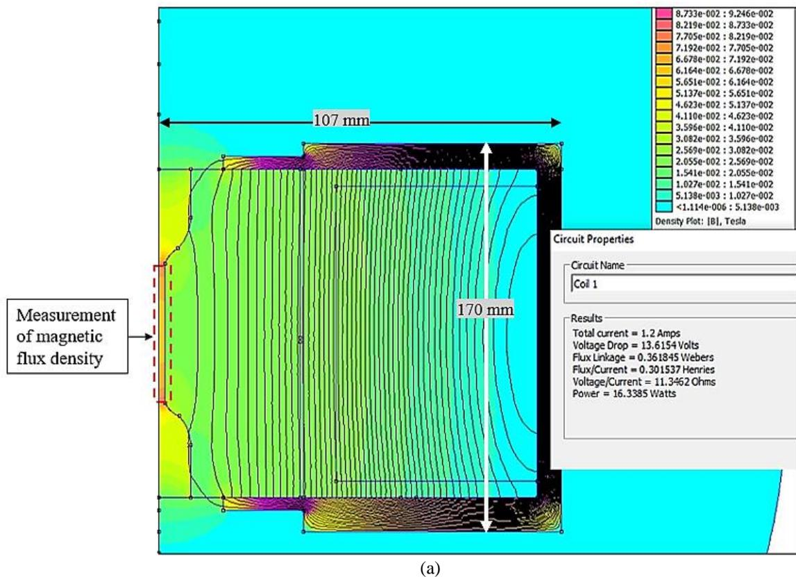
Figure 3. (a) FEMM simulation for 1.2 Amps with the area of magnetic flux measurement
