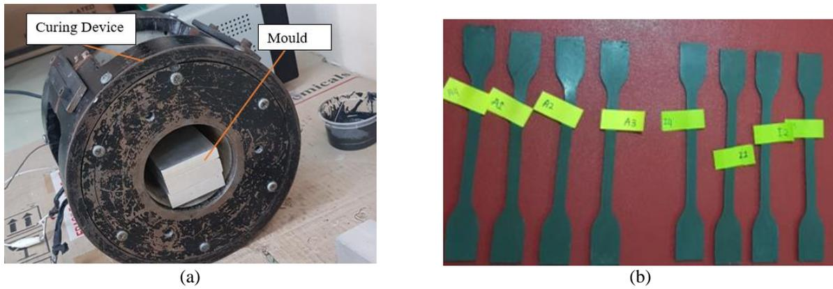
Figure 2. (a) Electromagnetic Curing device (b) MRE sample produced by the mold.
