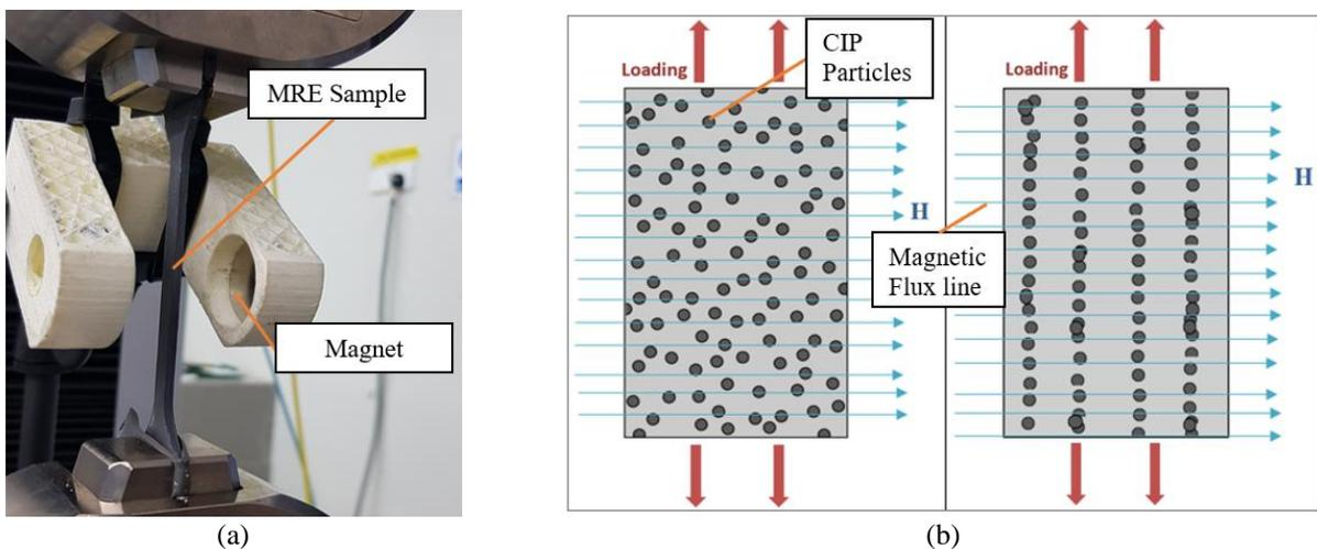
Figure 4. Tensile testing (a) Set-up configuration with magnet (b) Schematic of Isotropic (left) and Anisotropic (right) tensile testing configuration for 'ON' condition
