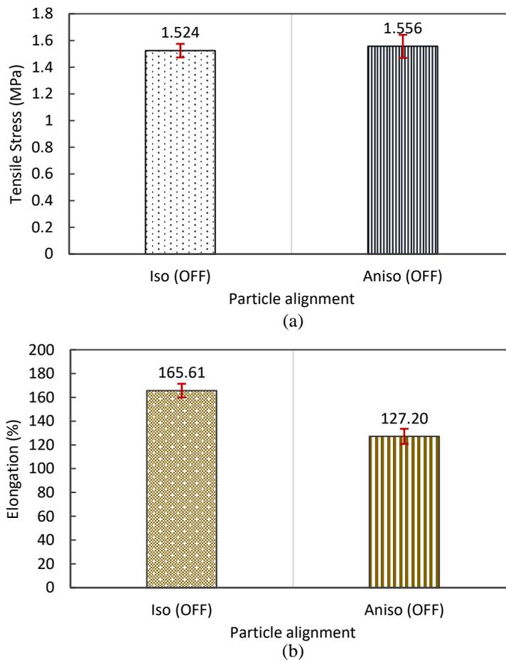
Figure 5. Isotropic vs Anisotropic (a) OFF-state Tensile Stress (b) OFF-state elongation
