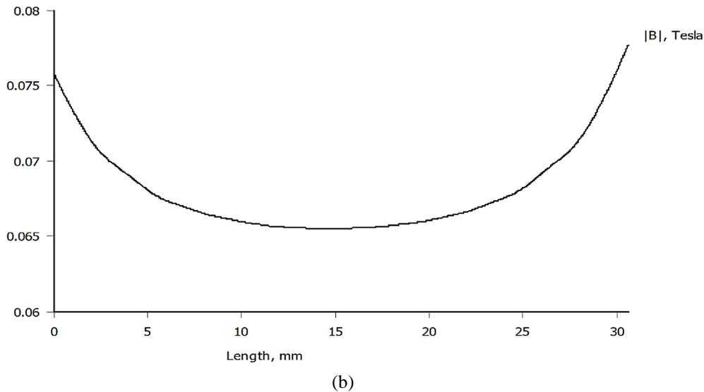
Figure 3. (cont.) (b) Magnetic flux density plot along the gauge length
