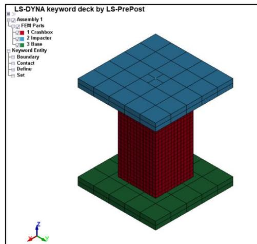
Figure 2. Quasi-static element model
