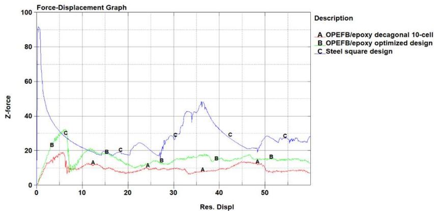
Figure 8. Force-displacement graph of steel and OPEFB/epoxy crash box
