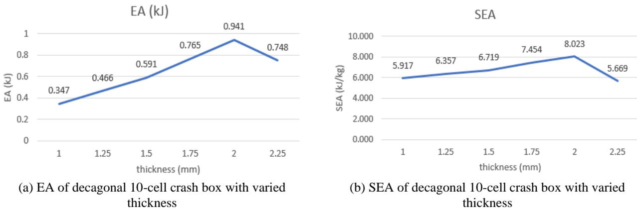
(a) EA of decagonal 10-cell crash box with varied thickness (b) SEA of decagonal 10-cell crash box with varied thickness
