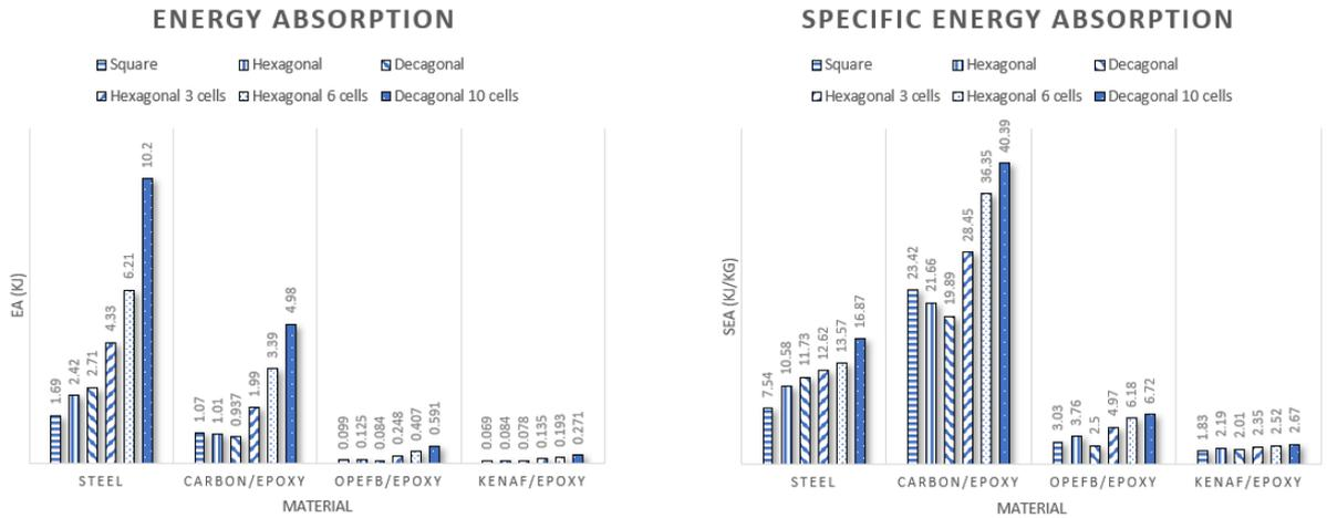
(a) EA of different materials using different designs (b) SEA of different materials using different designs
