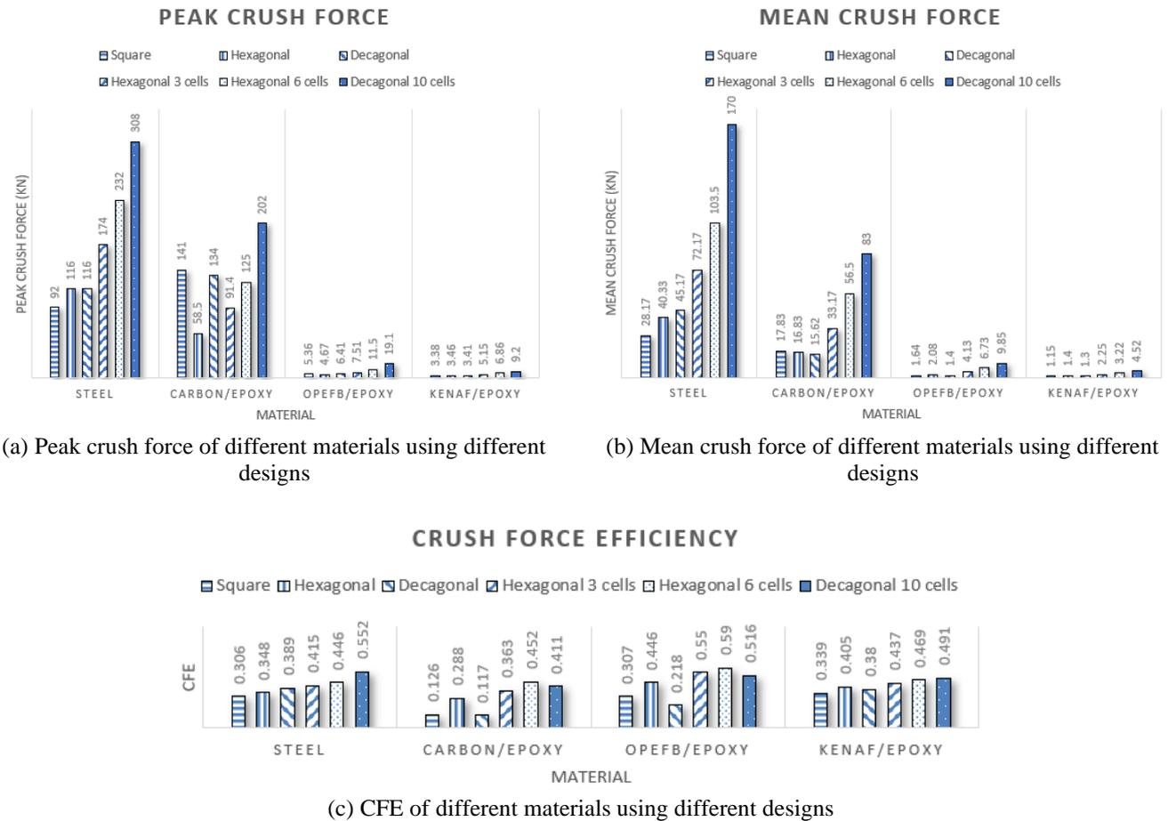
(a) Peak crush force of different materials using different designs (b) Mean crush force of different materials using different designs (c) CFE of different materials using different designs
