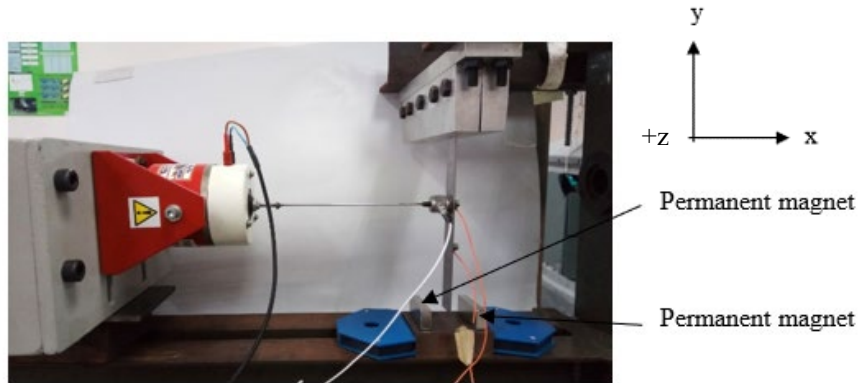
Figure 1. Experimental setup for linear and nonlinear modal analysis
