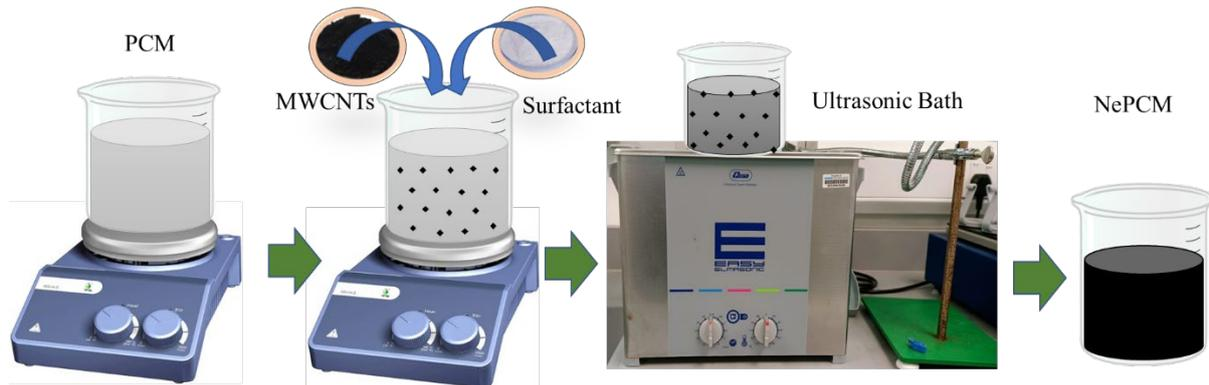
Figure 1. Schematic diagram of nanocomposite preparation method
