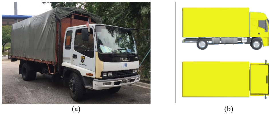
Figure 3. (a) ISUZU FSR two-axle SUT use for experiment, (b) virtual two-axle SUT model generated for simulation
