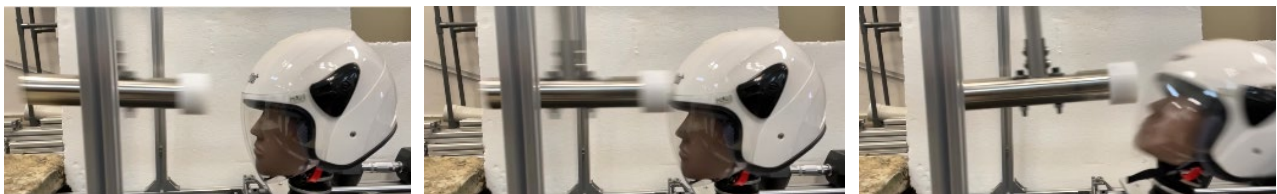
Figure 6. Sequence of pendulum impact when the pendulum cylinder struck the open-face helmet
