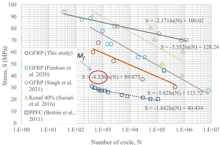
Figure 10. Comparison of the S–N curve of fabricated GFRP in this study to Ferdous et al. [14], Singh et al. [15], Suriati et al. [41] and Bettini et al. [42]
