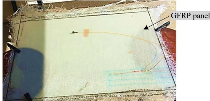
Figure 2. Fabricated GFRP panel and the fatigue test sample
