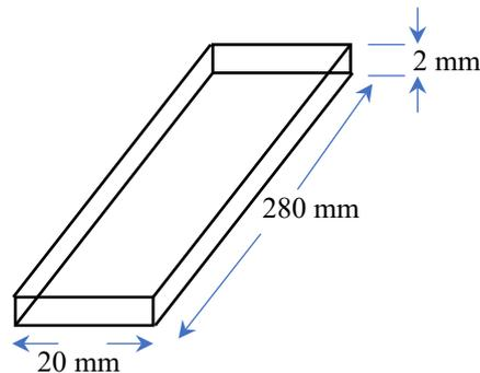
Figure 4. Fabricated GFRP fatigue test sample
