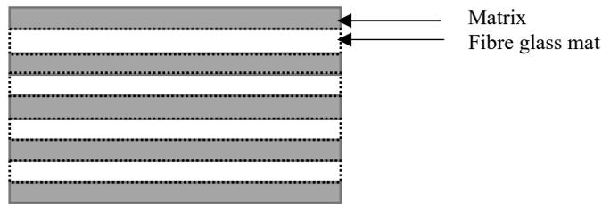
Figure 3. Schematic of GFRP composite that was fabricated from a combination of four layers of fibre mat and five layers of epoxy resin
