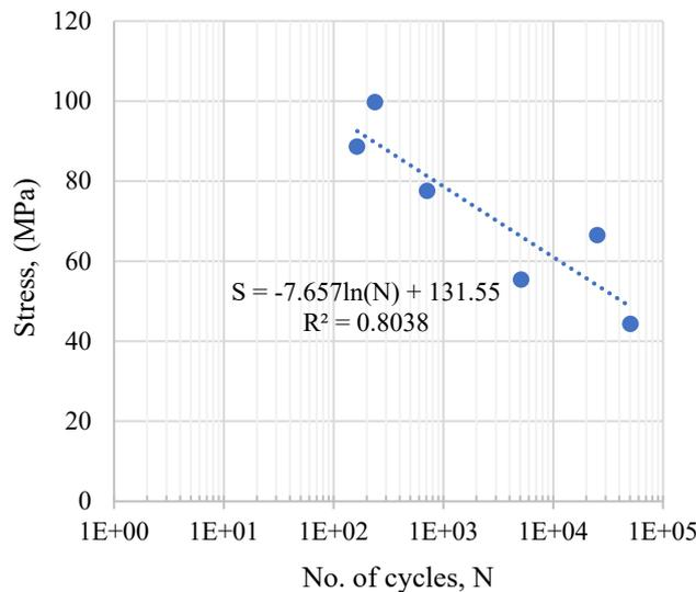
Figure 9. S–N curve of the fabricated GFRP
