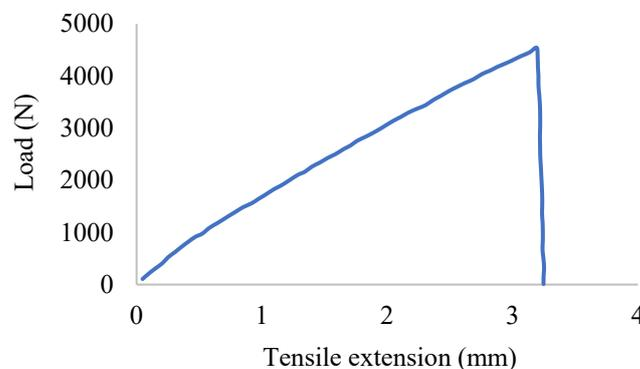
Figure 7. Load-extension curve of fabricated GFRP under tensile test
