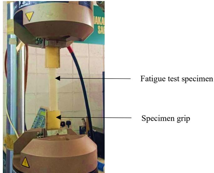
Figure 5. Tensile test setup of GFRP flat specimen
