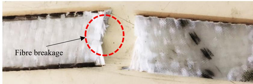
Figure 8. Fatigue failure on fabricated GFRP specimen at 60% stress level
