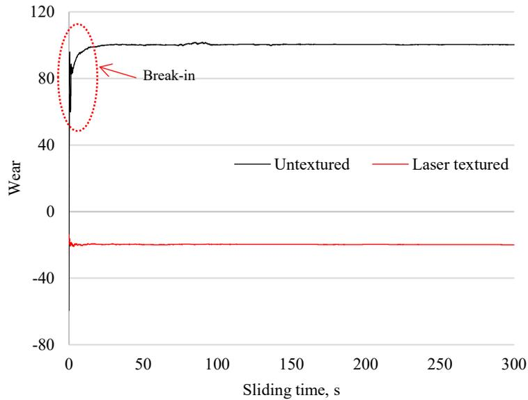
**Figure 1110.** The wear of untextured and laser-textured Ti6Al4V under oil lubricant conditions
