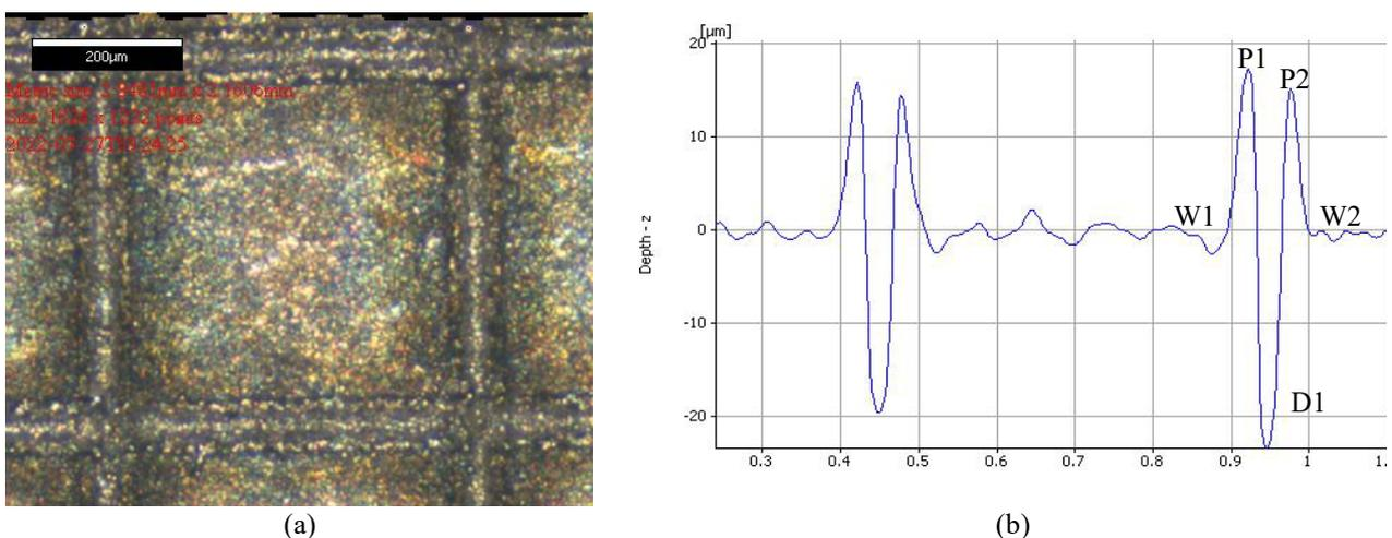
**Figure 1.** The LST of (a) grid-array pattern resulted on Ti6Al4V, and (b) surface profile of crater from laser textured
