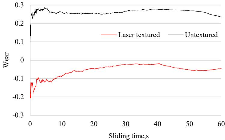
**Figure 109.** Wear behavior of untextured and laser-textured Ti6Al4V under dry sliding conditions
