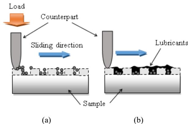
**Figure 1312.** A schematic diagram of active roles of surface texturing in frictional wear performance of (a) dry sliding condition, and (b) lubrication condition capturing friction debris
