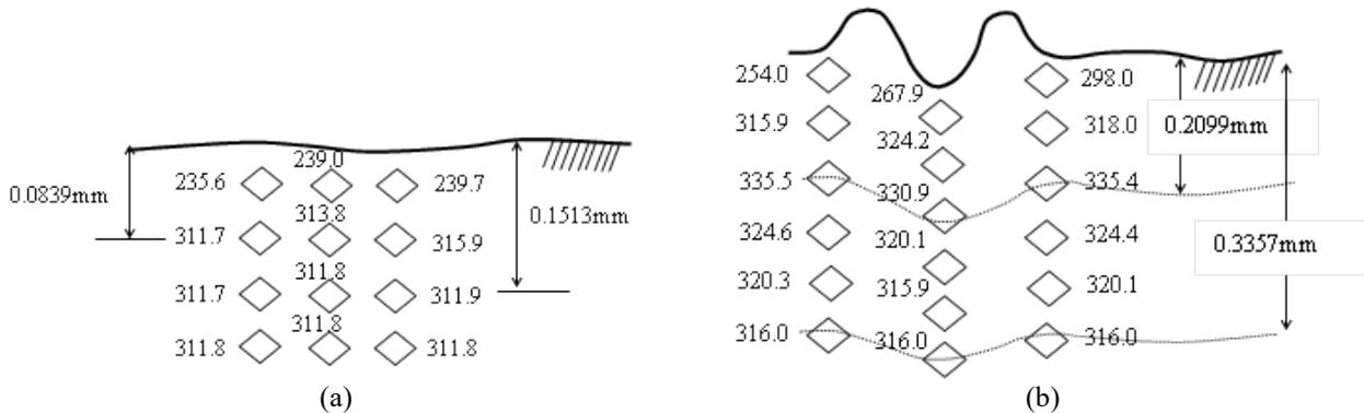
**Figure 54.** The microhardness value from Vickers hardness tester machine of (a) as received surface, and (b) laser textured surface
