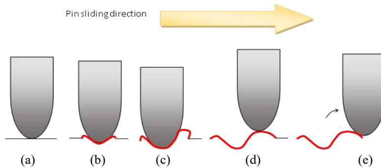
**Figure 87.** The volume displaced occurs, and the mark left on the pin is out from the wear track when the sliding speed increases
