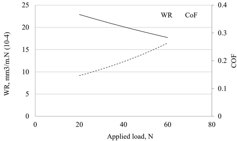
**Figure 76.** Effect of applied load on frictional wear behavior of the untextured Ti6Al4V surface
