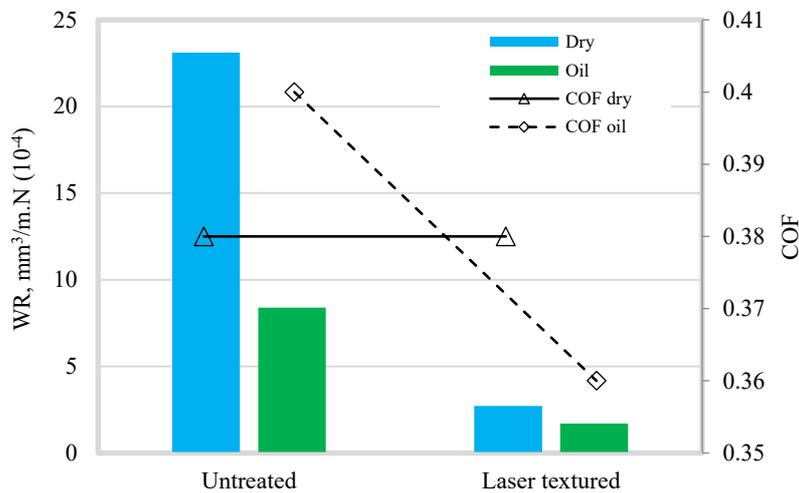
**Figure 1211.** The wear rate and COF of untextured and laser textured surface of Ti6Al4V under dry and oil lubrication test conditions for 20 N at 50 rpm with a sliding distance of 15 m
