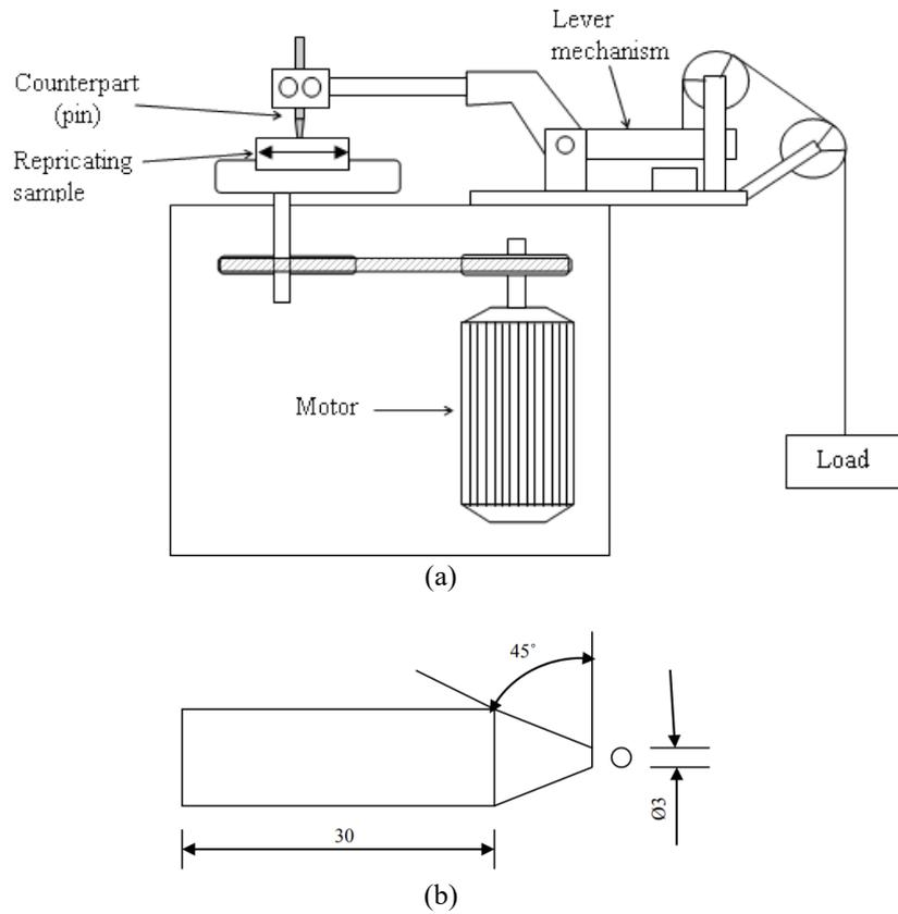
**Figure 21.** The schematic diagram of (a) pin-on-flat for frictional wear test and (b) standard dimension of pin for the test (all dimensions in mm)
