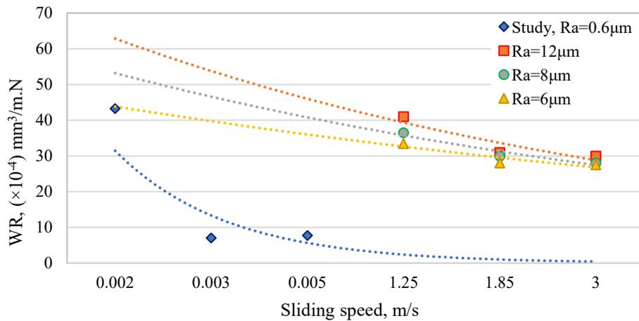
**Figure 65.** Effect of sliding speed on frictional wear behavior of the untextured surface compared to the study by Al-Samarai et al. [14] of three Ra values; Ra=12 µm, Ra=8 µm, and Ra=6 µm
