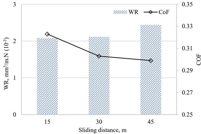
**Figure 98.** Effect of sliding distance on frictional wear behavior of the untextured Ti6Al4V
