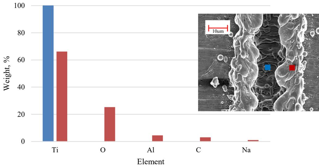
**Figure 32.** The result of SEM-EDX of laser textured Ti6Al4V on two different laser spots before the wear sliding test
