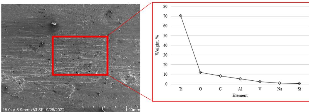
**Figure 43.** The result of SEM-EDX of untextured Ti6Al4V after sliding wear test indicates the formation of oxidation
