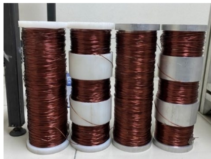
Figure 10. Cylindrical tube with copper coil winding
