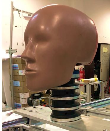
Figure 2. Hybrid III headform and neckform
