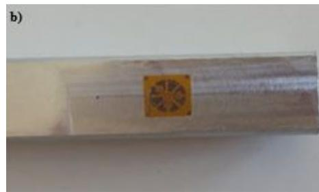
(b) strain-gage application on surface, and
