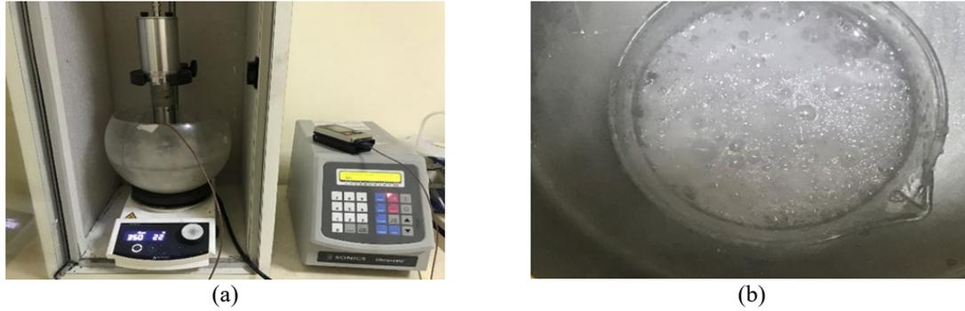
Figure 1. Nano alumina and epoxy resin suspension mixing process, (a) UDMM, (b) vacuum chamber degassing process
