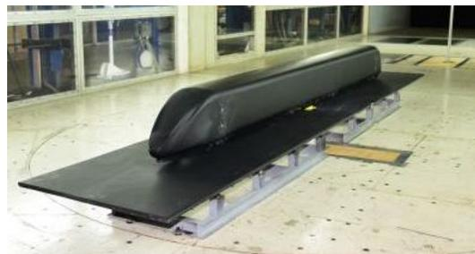
**Figure 12.** Wind tunnel test of HST scaled-model
