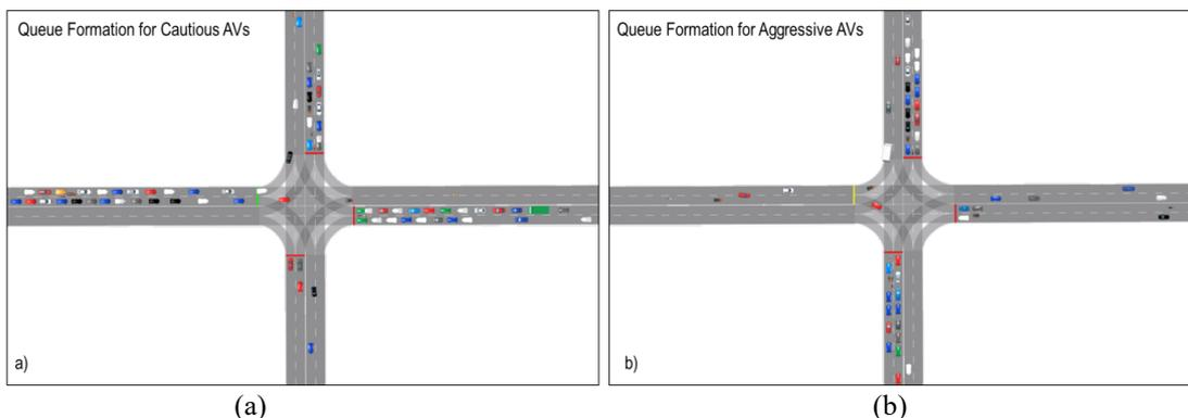
**Figure 10.** Queue formation for two vehicle compositions containing; (a) cautious AVs and (b) aggressive AVs
