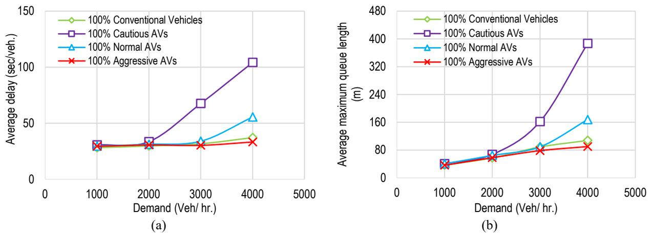
**Figure 6.** Impact of different types of vehicles on (a) average delay and (b) average maximum queue length
