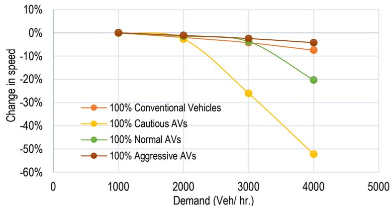
**Figure 7.** Impact of different types of vehicles on speed
