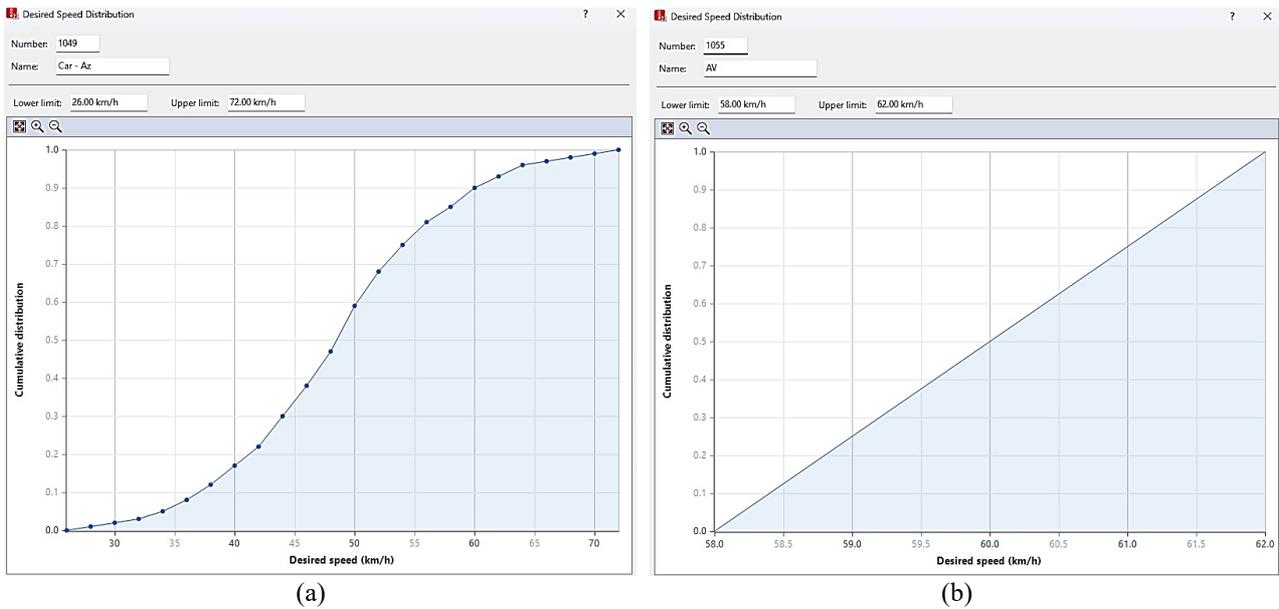
**Figure 4.** Desired speed distributions for different driving logics; (a) conventional car, (b) AV
