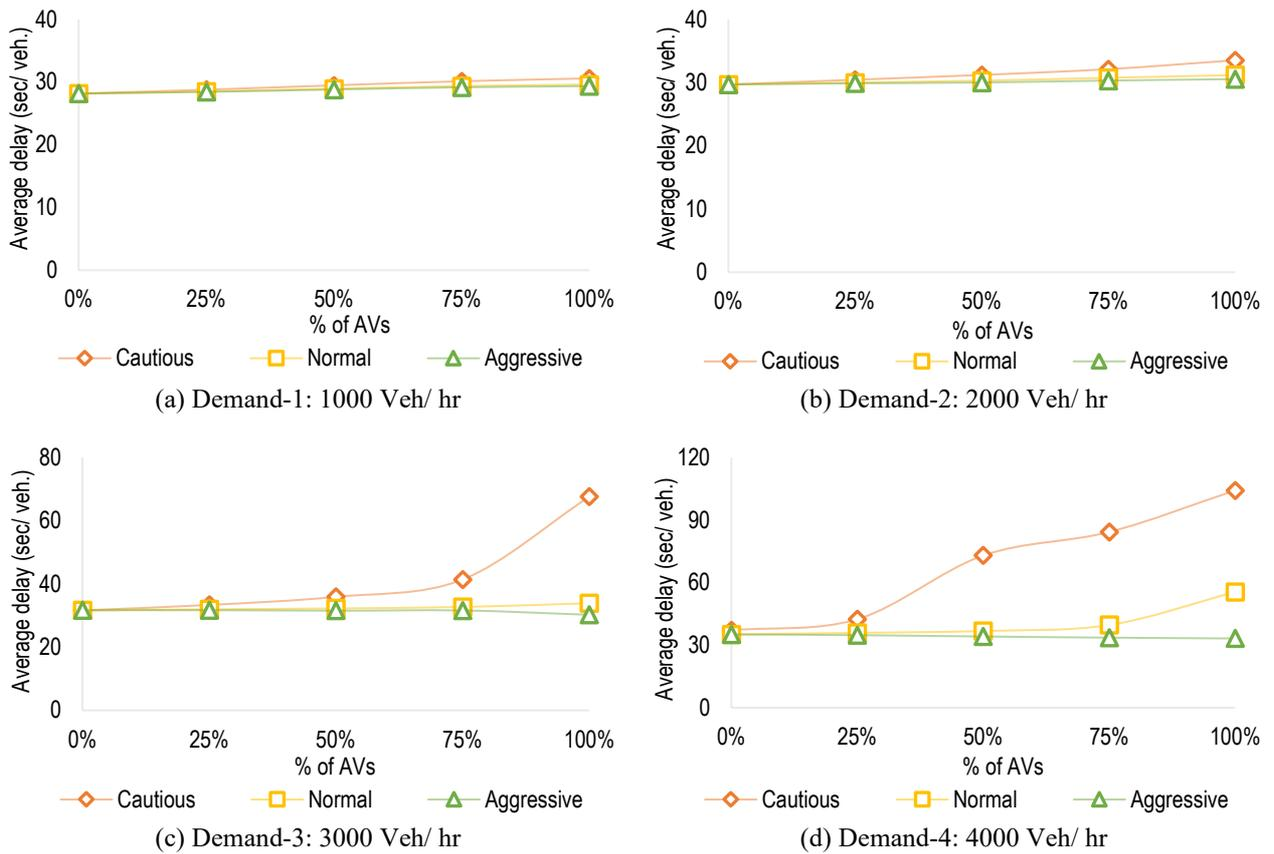
Figure 8. Impact of varying penetration rates of cautious, normal and aggressive AVs on average delay at four demand levels
