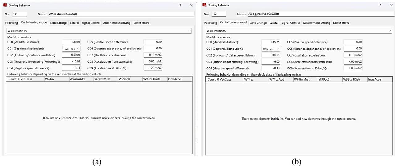
**Figure 5.** Car-following parameter setting for two driving logics; (a) cautious AV, (b) aggressive AV
