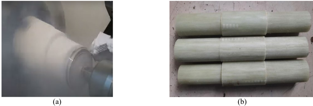
Figure 7. EGFRP cryogenic (a) machining and (b) machined samples
