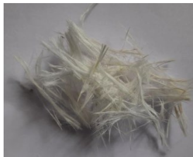
Figure 6. Buckling and bending failure of fibres
