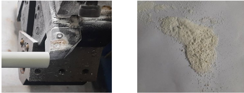
Figure 4. Powder forms of chips in machining operation
