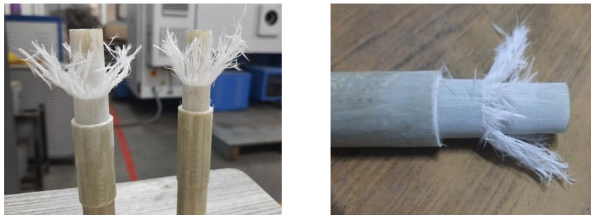
Figure 5. Fiber pullout under dry machining condition
