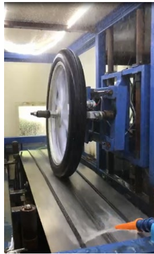
Figure 9. Water draining on the runway in front of the rolling tire
