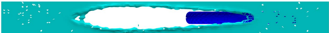
Figure 20. Water film on the road surface spreads by rolling tires with different inflation pressures at a velocity of 90 km/hr
