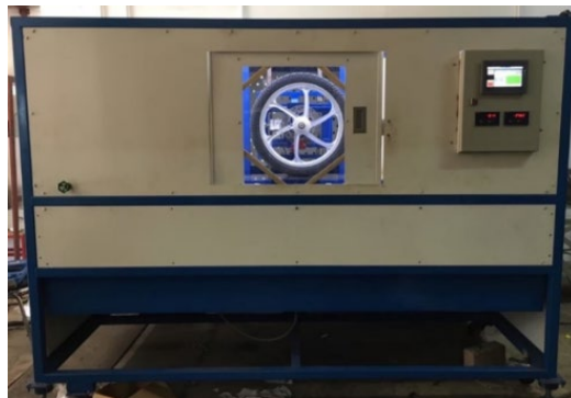
Figure 7. The hydroplaning testing machine invented for motorcycle tires
