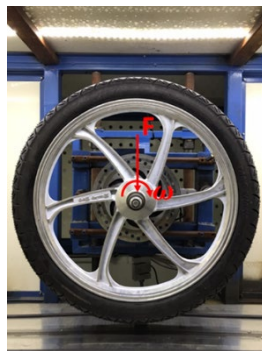
Figure 8. Installation of a motorcycle tire at the machine arm
