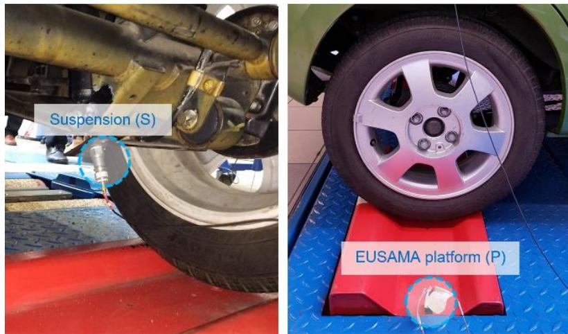
Figure 6. View of accelerometers location
