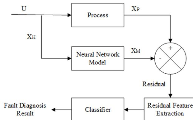
**Figure 4.** Block diagram of the proposed fault detection system
