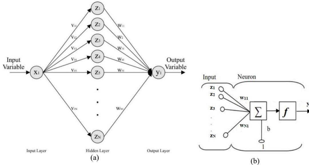
**Figure 3.** (a) ANN model structure and (b) a neuron in the output layer
