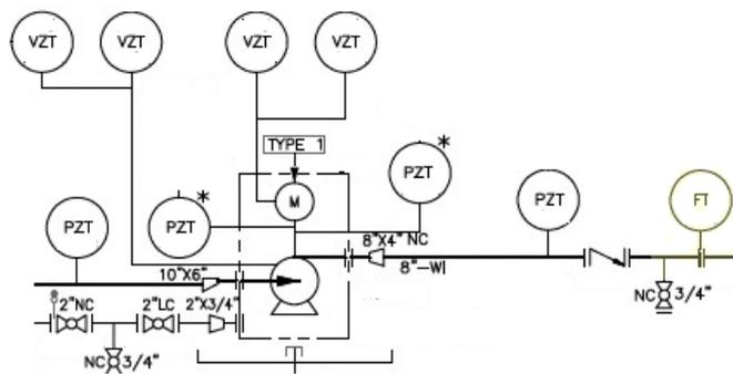
**Figure 7.** The P&ID of the installed pumps
