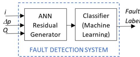
Figure 5. Pump condition monitoring system
