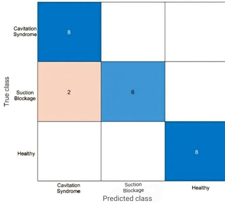
**Figure 13.** Confusion matrix with Support Vector Machine classifier testing
