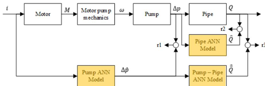
Figure 2. Residual analysis on centrifugal pump fault detection system
