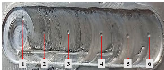
Figure 5. Location for hardness test points
