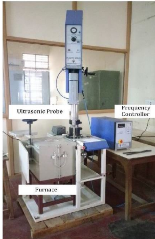
Figure 2. Experimental setup of ultrasonically assisted stir casting.
