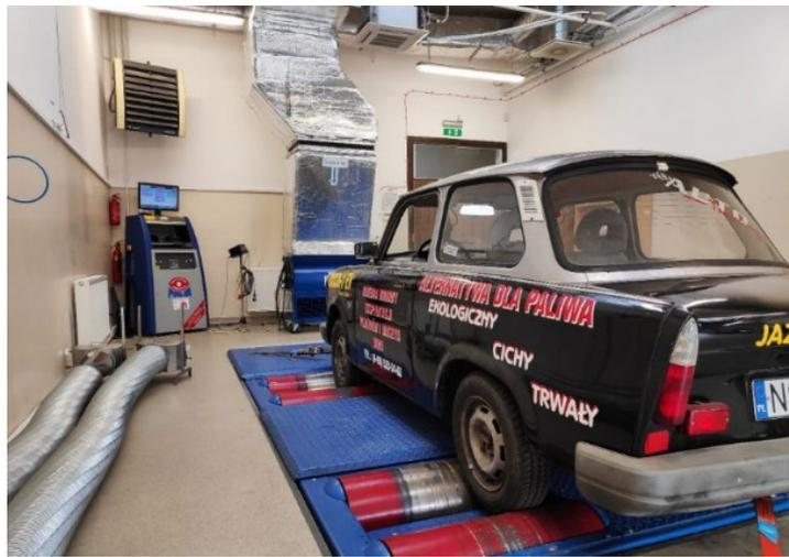
Figure 5. Traction tests of the EV on a MAHA LPS 3000 Chassis Dynamometer.
