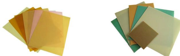
**Figure 1.** Glass fiber reinforced polymer laminates.
