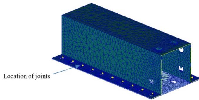
**Figure 2.** Finite element model of a top-hat beam with welded joints.
