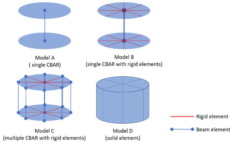
**Figure 1.** Illustration of spot weld finite element models.
