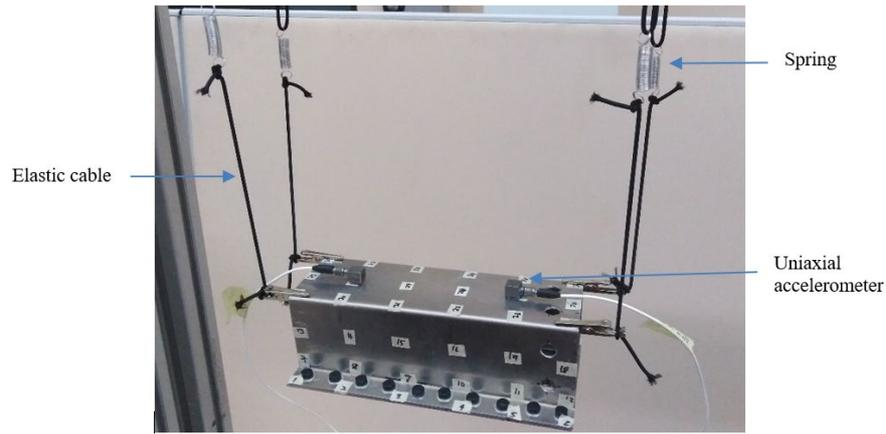
**Figure 3.** Tested top-hat structure under free-free boundary condition.
