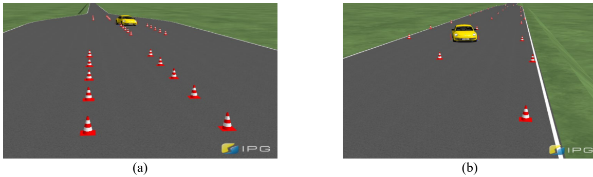
Figure 8. (a) Double lane change test and (b) slalom test at 80 km/h.
