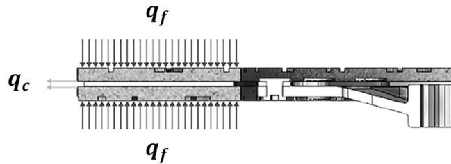
Figure 3. Loads and boundary conditions for the thermal model.
