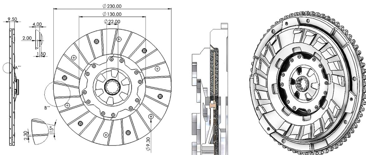
**Figure 1.** Dimensions and features of the clutch geometry.
