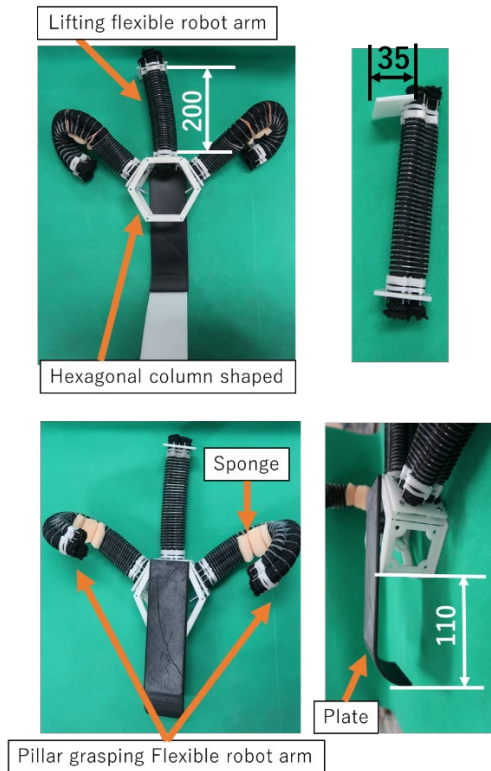
Figure 15. Appearance of the tested automatic ladder climbing robot.
