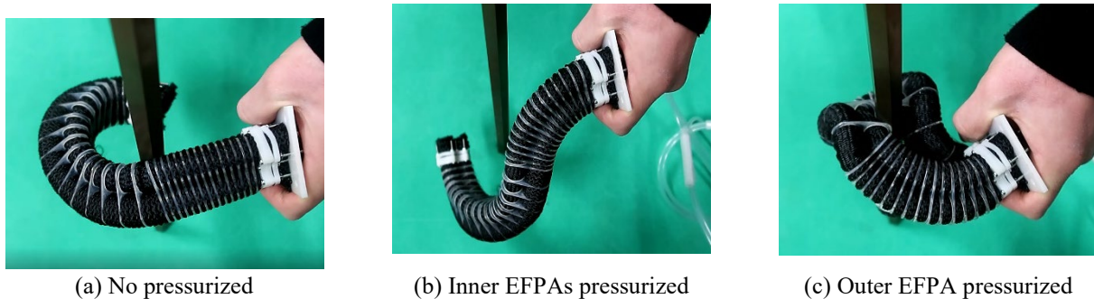
Figure 14. Operation of the tested robot arm using two on/off valves.
