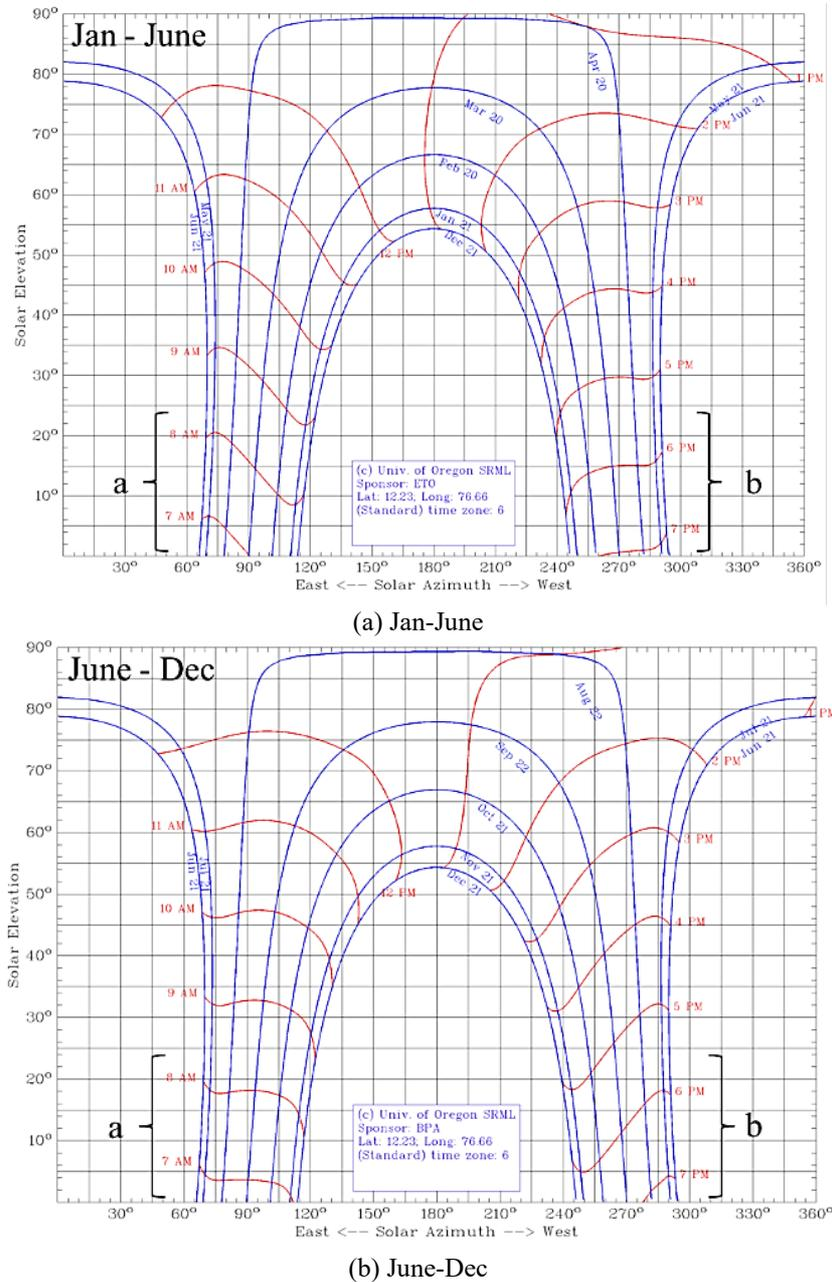
Figure 9. Sun Path chart and glare occurrence in PV array [29].
