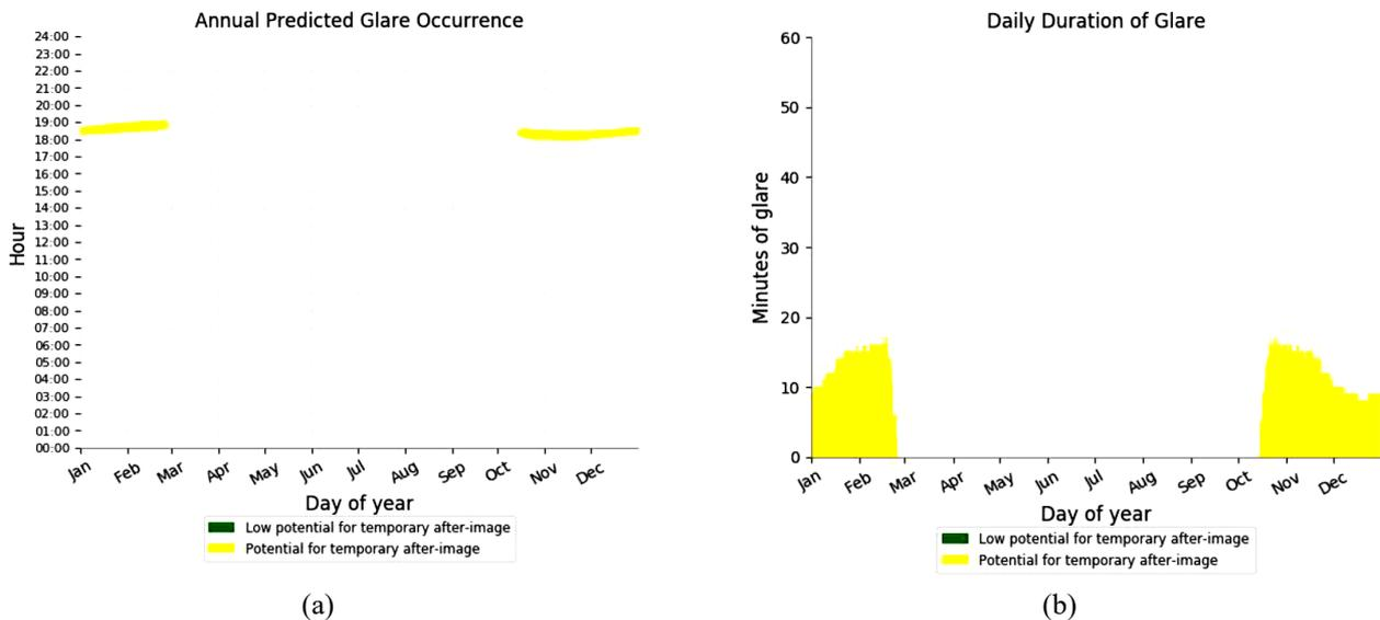
**Figure 5.** Variation of (a) glare duration occurrence and (b) duration from fixed-tilt solar PV array for ATC.
