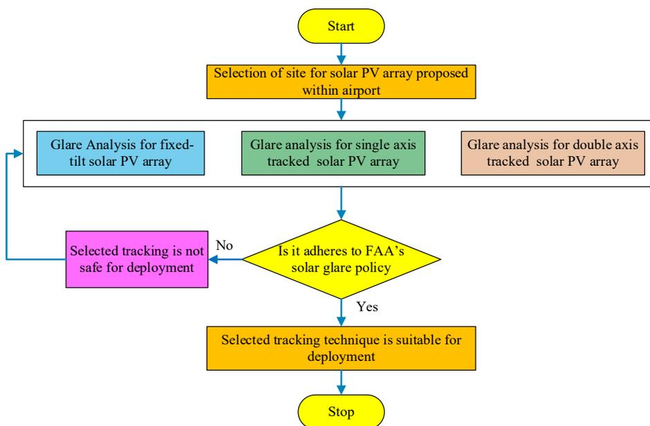
Figure 4. Methodology of suitability analysis of solar tracking based on glare.
