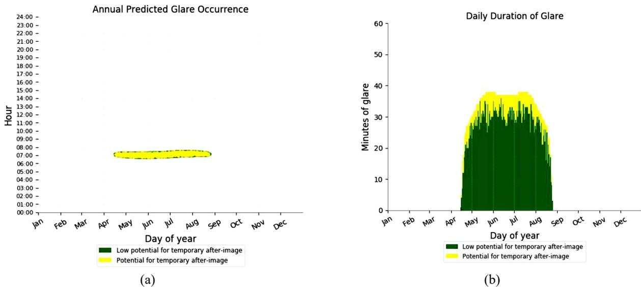
Figure 8. Variation of glare (a) duration occurrence and (b) duration from dual-axis solar PV array for ATC.
