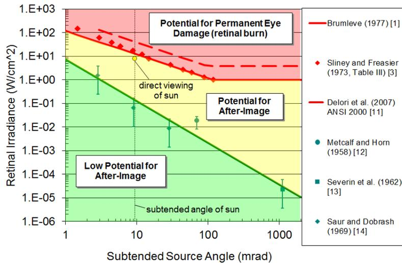
Figure 3. A sample solar glare hazard plot.
