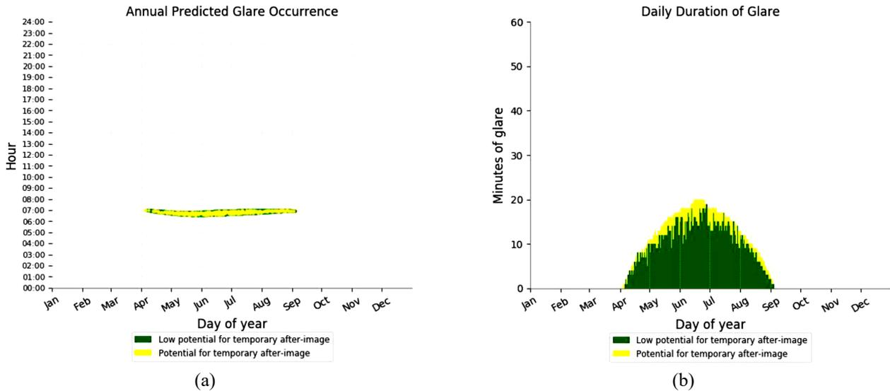
Figure 6. Variation of glare (a) duration occurrence and (b) duration from dual axis solar PV array for flight path 1.
