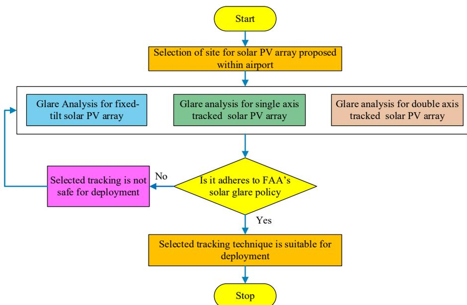
Figure 4. Methodology of suitability analysis of solar tracking based on glare.
