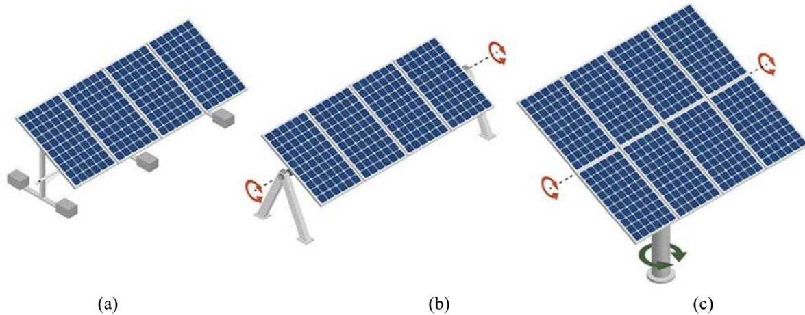
**Figure 1.** Different types of solar PV array based on its tracking of sun's movement, (a) fixed-tilt, (b) single axis tracker, and (c) dual axis tracker [5].
