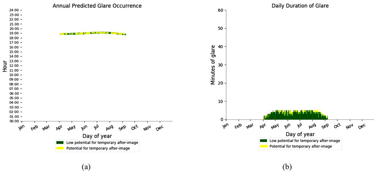
Figure 7. Variation of glare (a) duration occurrence and (b) duration from dual axis solar PV array for flight path 2.
