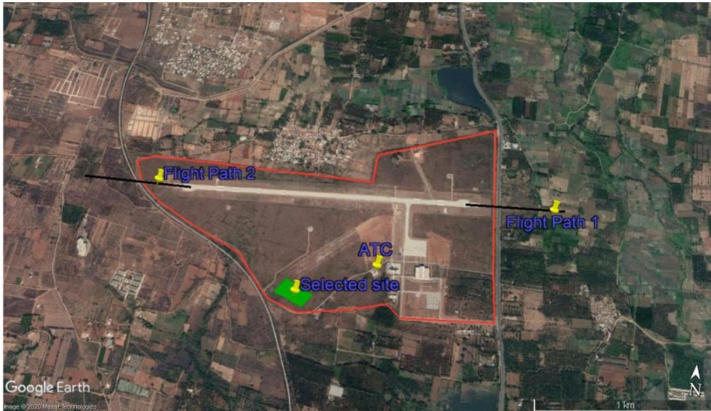
**Figure 2.** Location of the proposed solar PV array and sensitive observation points.
