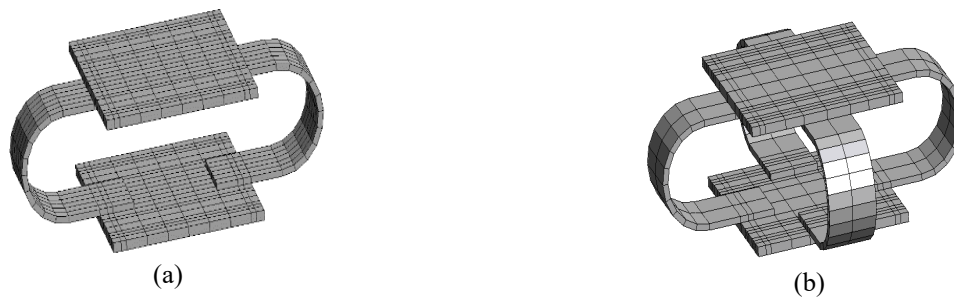
Figure 5. Variation of configurations of U-shaped steel damper (a) Model_21: A pair of U-steel plate configurations on one side of the damper, representing unsymmetrical damper, (b) Model_22: Two-pairs of U-steel plate configurations on both sides of the dampers, representing symmetrical damper.
