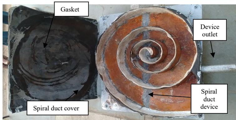
**Figure 7.** Device cover with gasket.
