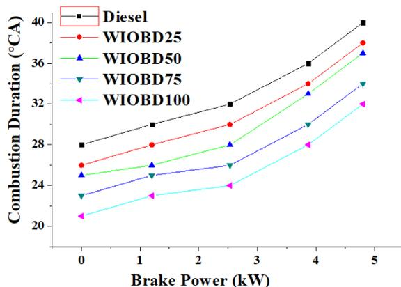
Figure 12. Combustion duration vs BP for WIOBD-diesel blends.
