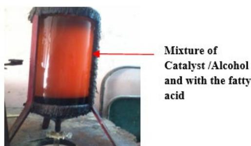
(a) reaction between the mixture of catalyst/alcohol and with the fatty acid (triglycerides)
