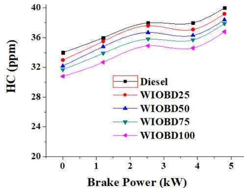
**Figure 15.** HC emission vs BP for different blends of WIOBD-biodiesel.
