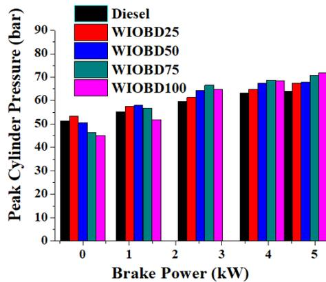
**Figure 9.** Peak Cylinder pressure vs BP for diesel and WIOBD-blends.
