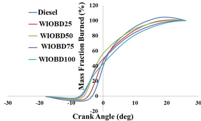
Figure 13. MFB vs crank angle for various blends of WIOBD-diesel at full load.
