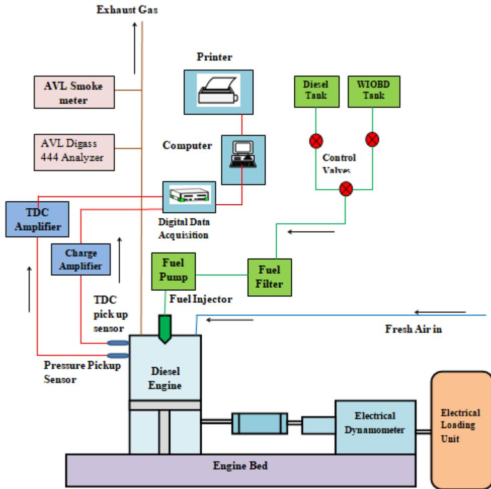
Figure 3. Experimental setup of the diesel engine along with the instrumentation.
