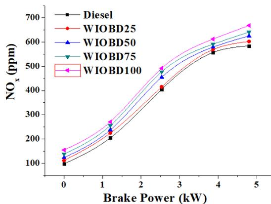
**Figure 16.** NO<sub>x</sub> emission vs BP for different blends of WIOBD-biodiesel.
