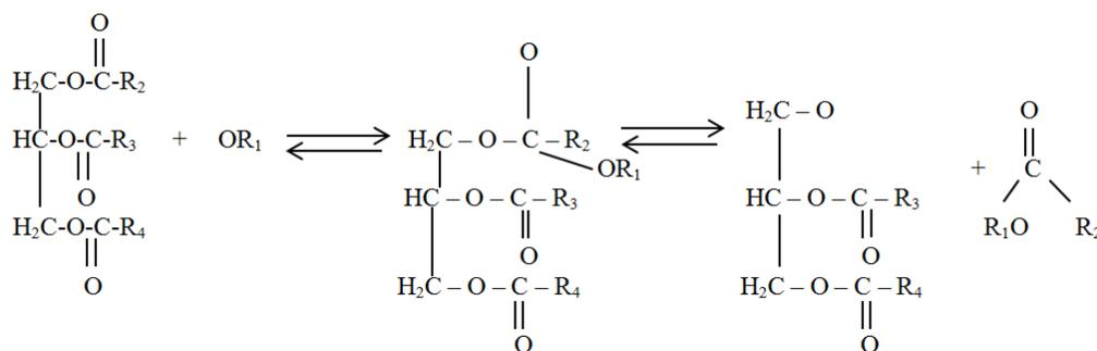
Figure 1. Biodiesel trans-esterification process.
