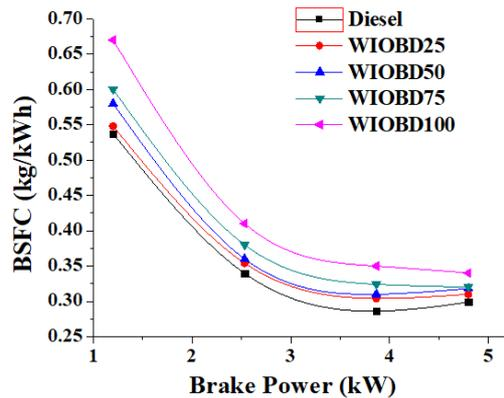
Figure 4. BSFC Vs BP for diesel and WIOBD-blends.
