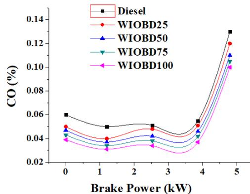
Figure 14. CO emission vs BP for different blends of WIOBD-biodiesel.
