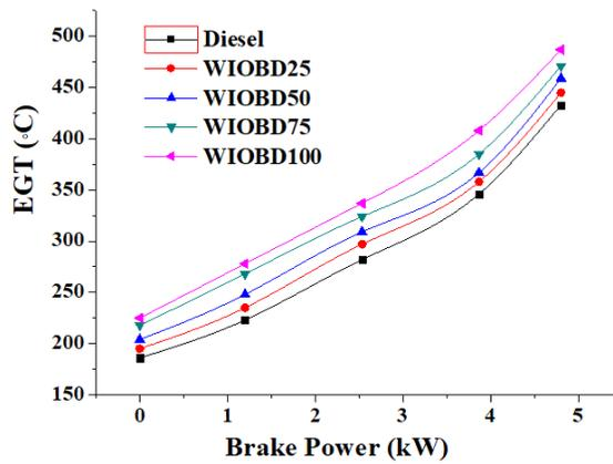
Figure 6. EGT Vs BP for diesel and WIOBD-blends.
