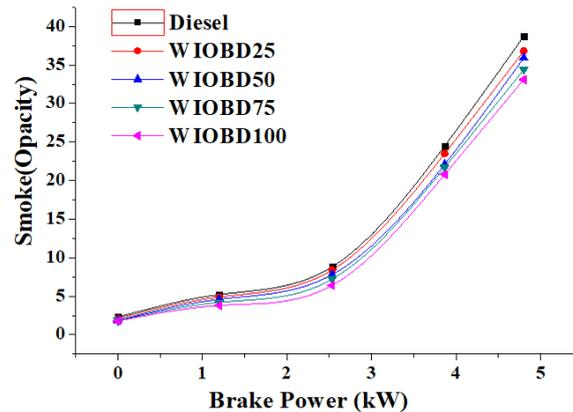
Figure 17. Smoke emission vs BP for various blends of WIOBD-biodiesel.
