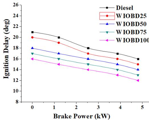
Figure 7. Ignition delay vs BP for diesel and WIOBD-blends
