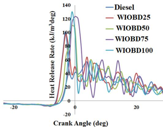
Figure 10. HRR vs crank angle for diesel and WIOBD-blends.
