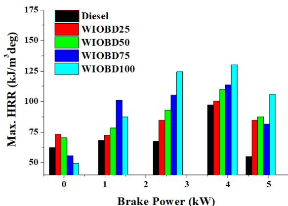
Figure 11. Maximum HRR vs BP for WIOBD-diesel blends.
