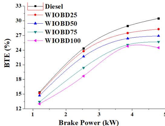
Figure 5. BTE Vs BP for diesel and WIOBD-blends.
