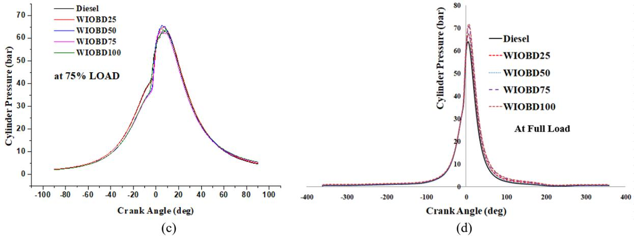
**Figure 8.** Cylinder pressure vs. crank angle for diesel and WIOBD-blends at different loads.
