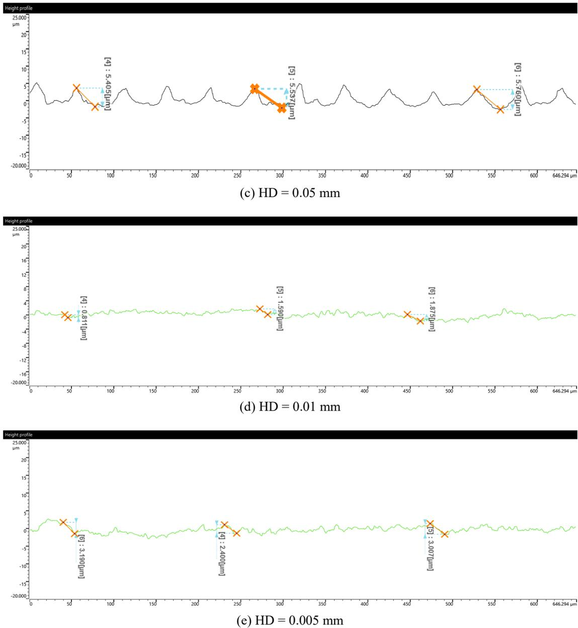
**Figure 4.** Profile measurement for the textured surface of different hatch distances.
