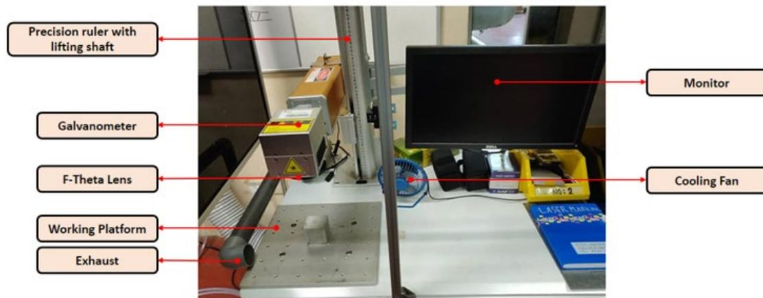
**Figure 1.** Laser marking machine apparatus for laser surface modification.
