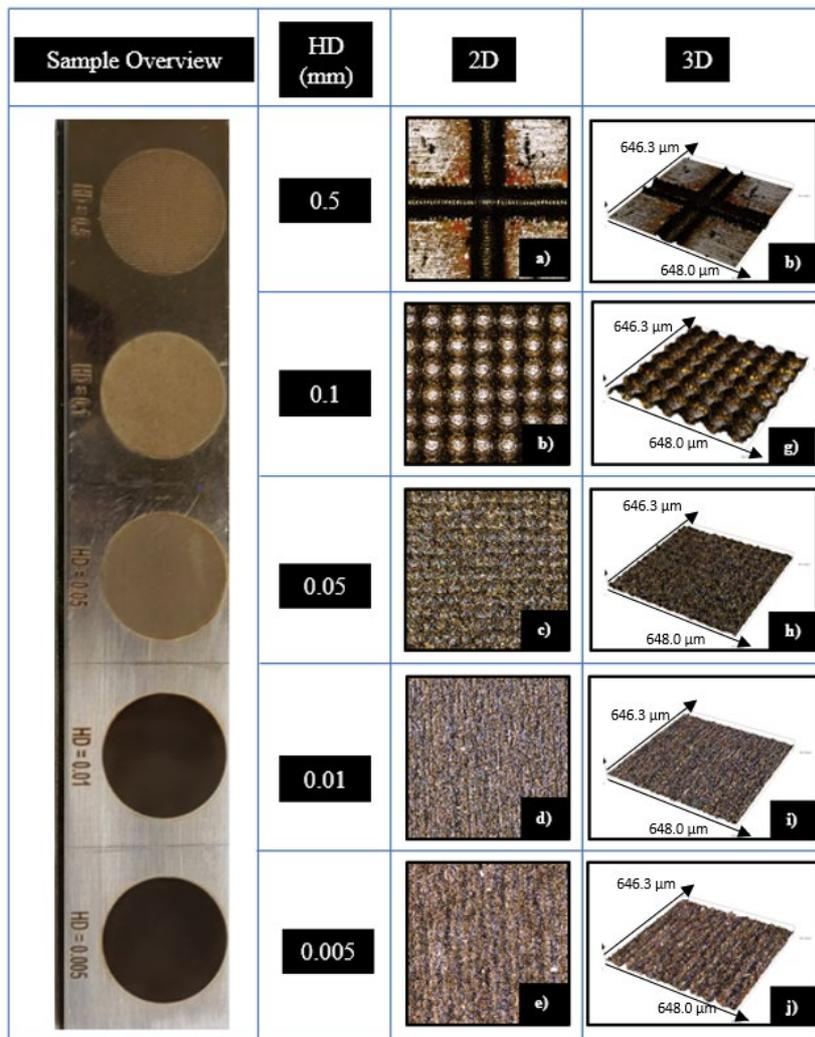
**Figure 2.** Overview of 3D, 2D of sample optical image from laser scanning on each LSM sample with different hatching distance from 0.5 to 0.005.
