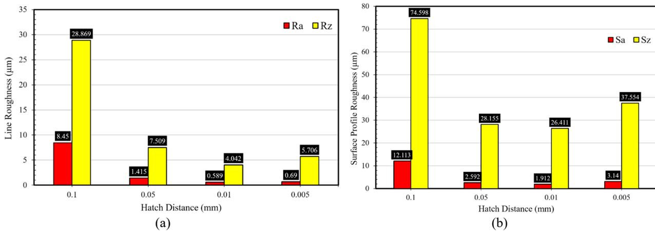
**Figure 5.** (a) Line roughness and (b) surface profile roughness for the sample with hatch distance of 0.1, 0.05, 0.01, and 0.005 mm.
