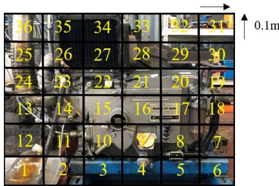
Figure 3. Gridding of a noise source.
