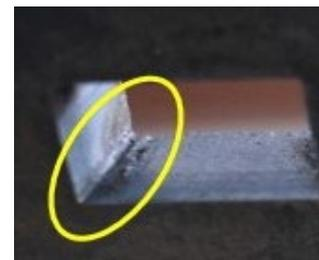
(c) Damages of corner edge in a few holes
