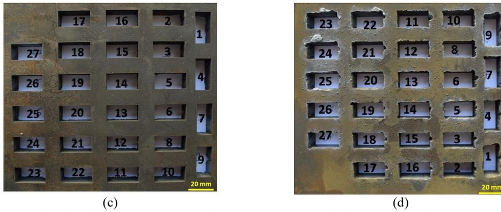
**Figure 1.** Position of holes from the (a) top view of the untreated plate, (b) bottom view of the untreated plate, (c) top view of HT plate and (d) bottom view of HT plate.
