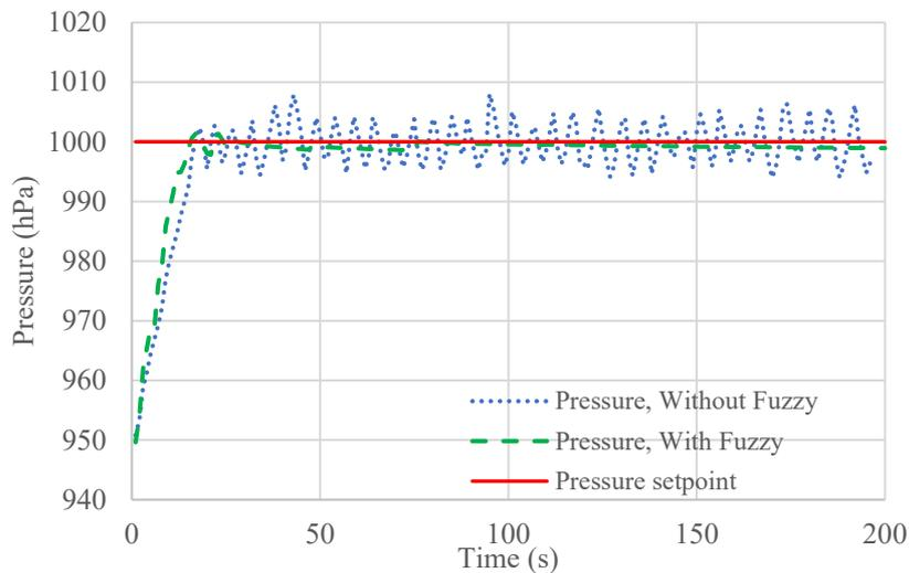
Figure 6. Time versus pressure for the pressure stability test.
