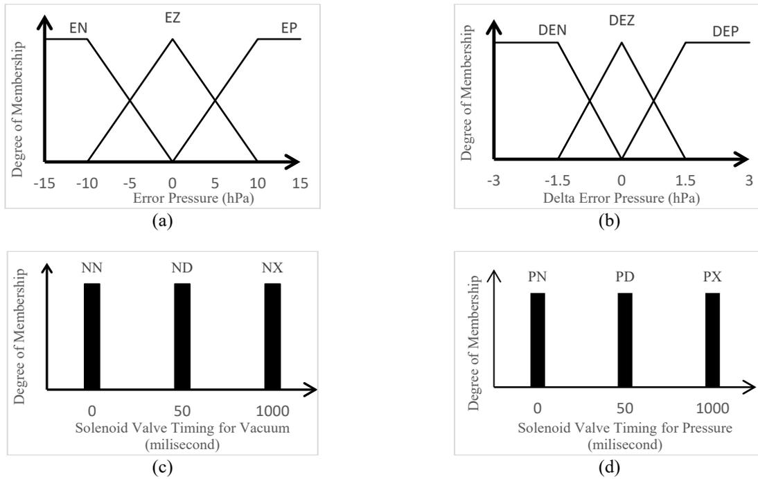
Figure 5. Fuzzification process. (a) input (error), (b) input (delta error), (c) output (vacuum), (d) output (pressure).
