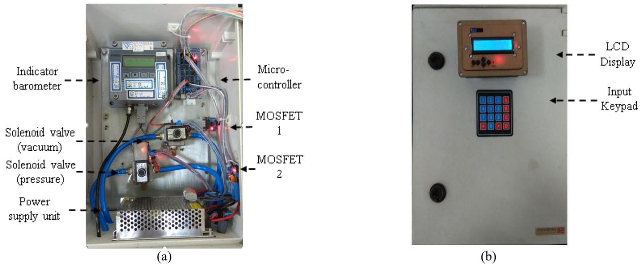
**Figure 3.** (a) Inside view and (b) front view of automatic pressure chamber controller.
