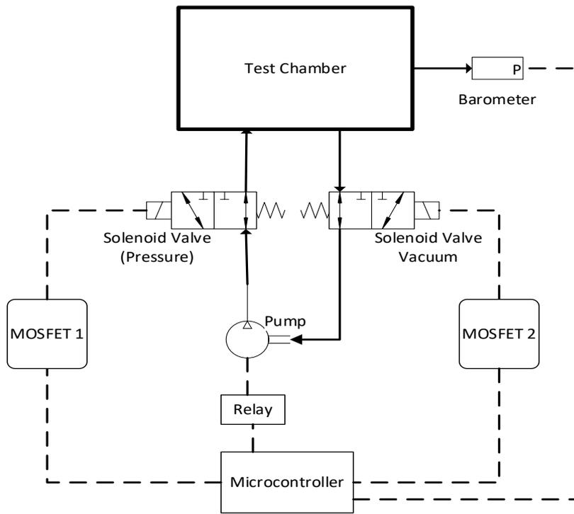
**Figure 2.** Schematic diagram of fuzzy logic controller for pressure sensor calibration chamber.
