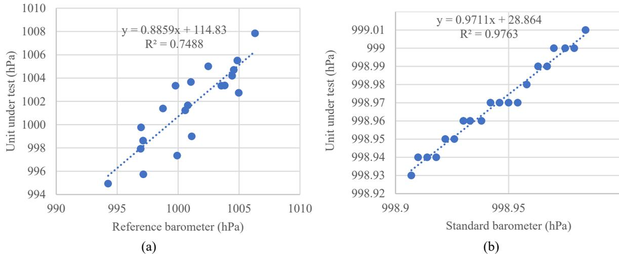
**Figure 7.** Calibration data (a) without fuzzy logic and (b) using fuzzy logic.
