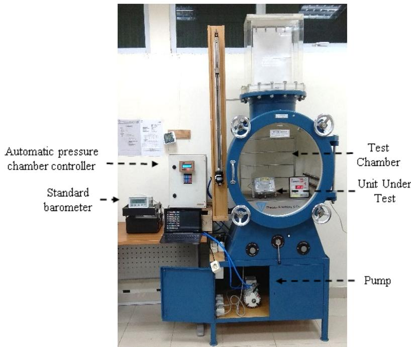
Figure 5. Calibration process.
