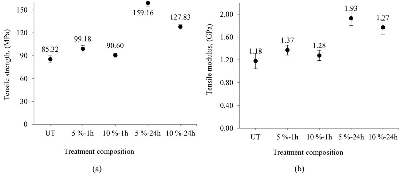
**Figure 8.** (a) Tensile strength and (b) tensile modulus of single-strand buri fibre untreated and alkaline treatment.
