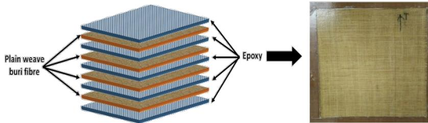
**Figure 3.** Staking sequence of woven buri fibre and epoxy composites.
