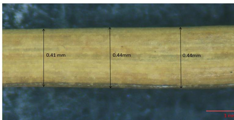
**Figure 5.** Image of the cross-sectional area and fibre width for single strand.
