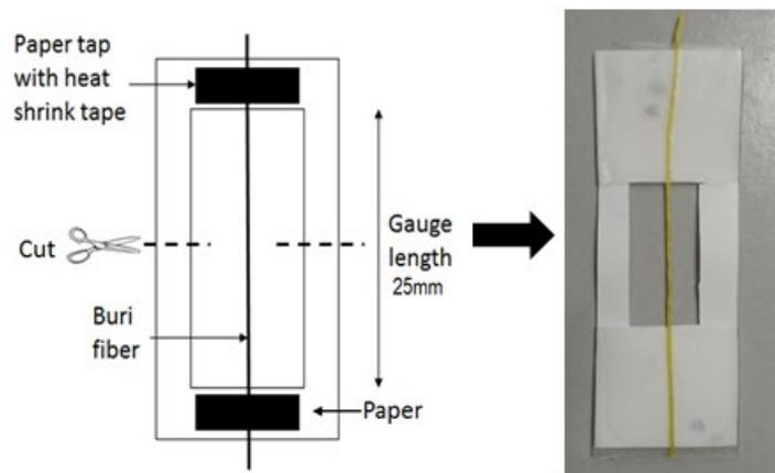
**Figure 4.** Buri strand fibre attached to a paper holder.
