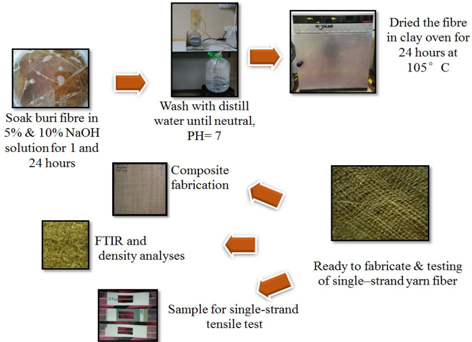
**Figure 1.** Process flow of alkali treatment of buri palm fibre.
