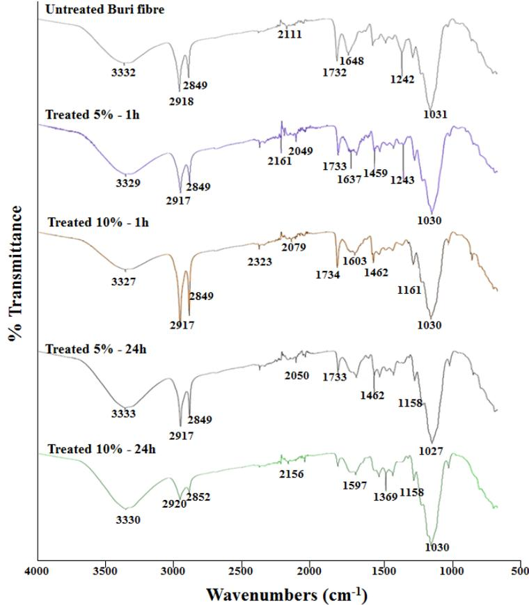
**Figure 7.** FTIR untreated buri fibre and treated spectrum of 5% - 1 h, 5% - 24 h, 10% - 1 h and 10% - 24 h.
