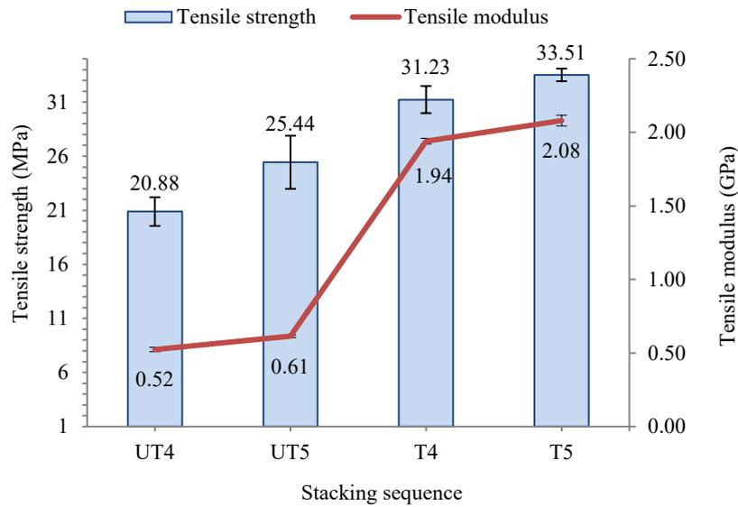
**Figure 9.** Tensile strength and tensile modulus of untreated and treated buri fibre stacking sequence composites.
