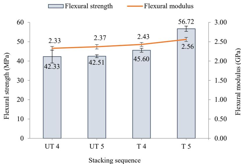
**Figure 11.** Flexural strength and flexural modulus of untreated and treated buri fibre stacking sequence composites.
