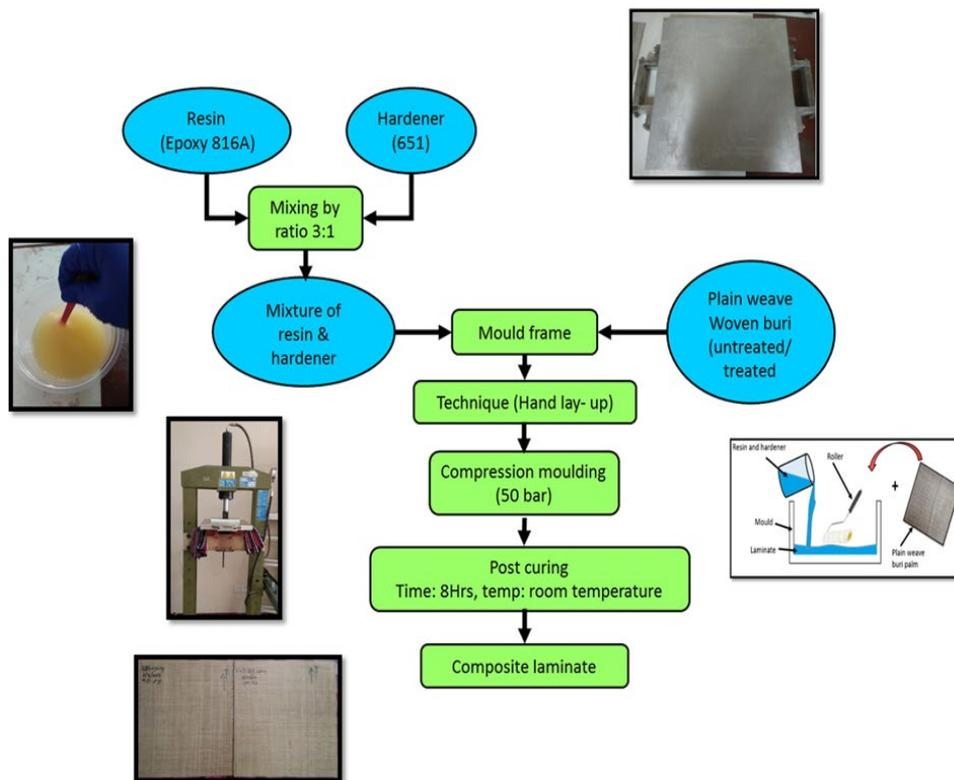
**Figure 2.** Process fabrication of woven buri palm fibre reinforced epoxy composites.
