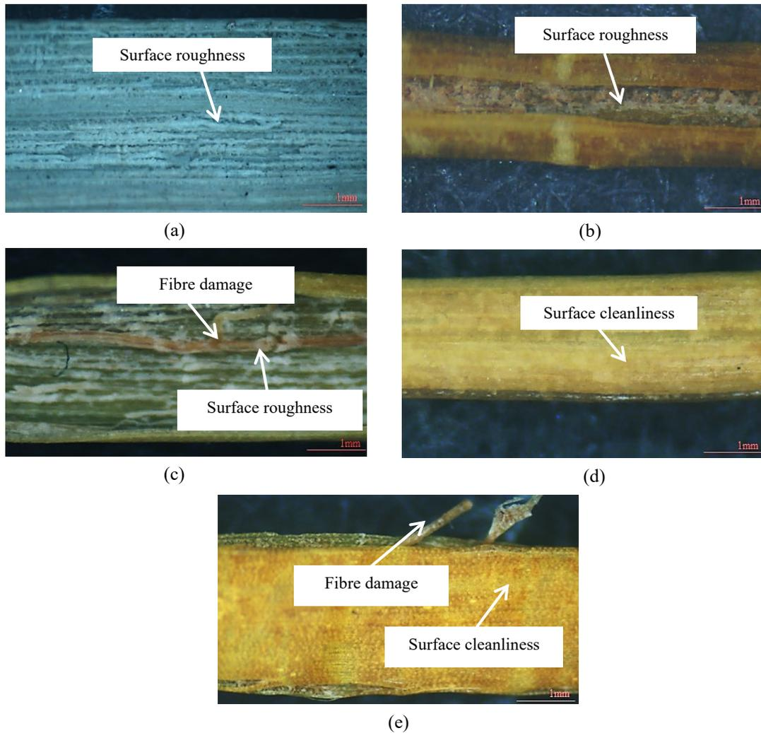
**Figure 6.** The physical appearance and effect of buri fibre after alkaline treatment under optical microscopy: (a) untreated strand fibre, (b) 5% NaOH solution 1 h immersion, (c) 10% NaOH solution 1 h immersion, (d) 5% NaOH solution 24 h immersion, (e) 10% NaOH solution 24 h immersion.
