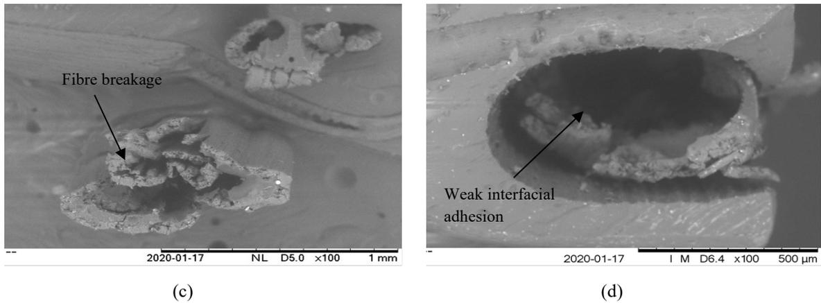
**Figure 10.** Tensile fracture specimen under SEM micrographs for (a) UT 4, (b) UT 5, (c) T4, and (d) T5.
