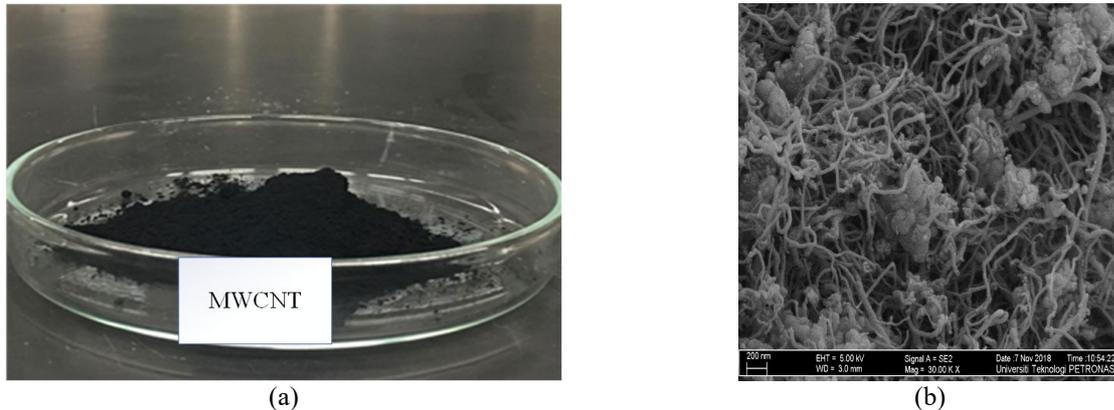
**Figure 1.** (a) Photograph of MWCNT nanoparticle (b) FESEM image of MWCNT nanoparticle at different magnitude.
