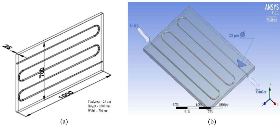
**Figure 2.** (a) Geometric model of the MCHS with external dimensions (b) CFD model of the MCHS with internal dimensions.
