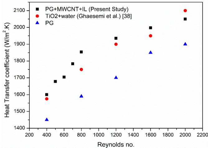
**Figure 7.** Heat transfer coefficient of the MCHS with different fluids at 0.5 wt.%.
