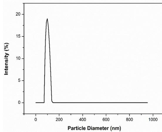
**Figure 5.** Particle size distribution of MWCNT nanoparticles dispersed in the base fluid.
