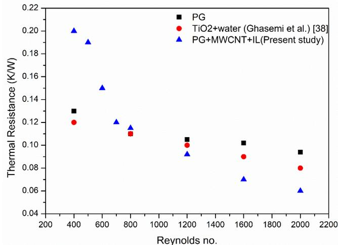
**Figure 8.** Thermal resistance of MCHS with different fluids at 0.5 wt.%.
