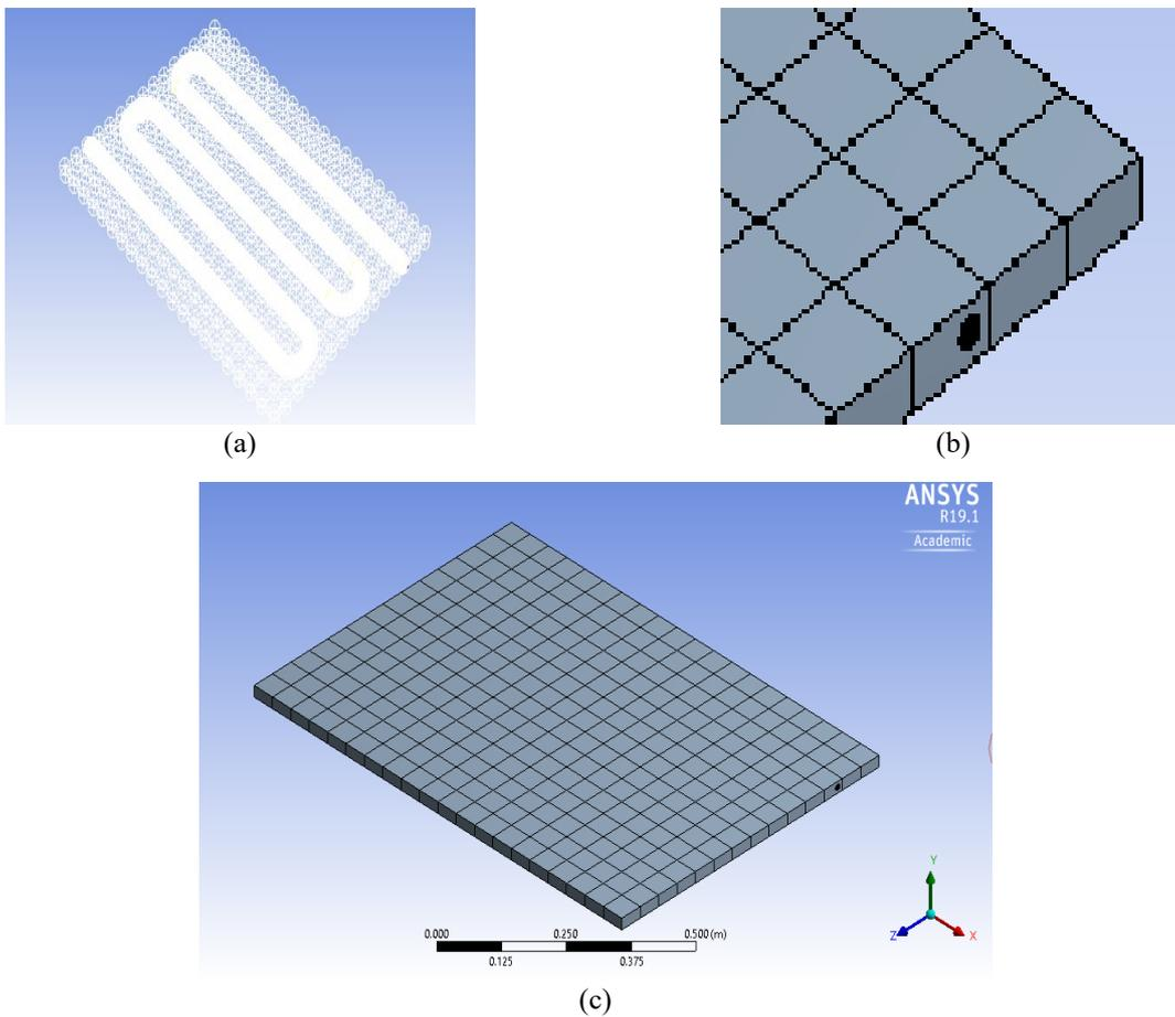
**Figure 3.** (a) Tube and heat sink mesh, (b) zoomed image of meshed MCHS and (c) total body mesh.
