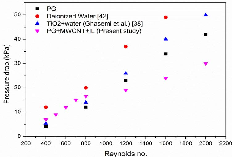
Figure 9. Pressure drop of MCHS with different fluids at 0.5 wt.%.
